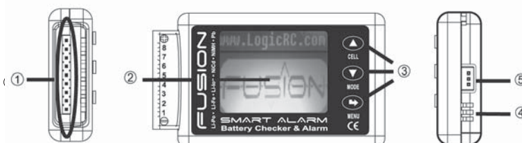
1. Input plug 2. LCD screen 3. Function button 4. Beep 5. Alarm port
