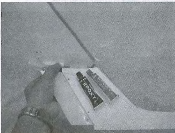
Glue the horizontal on the vertical using Epoxy.
