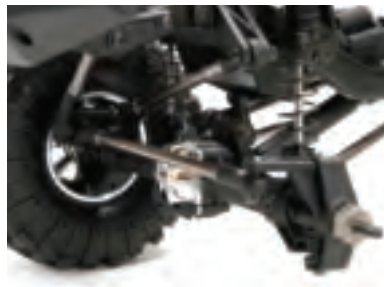
3-link panhard bar front suspension
