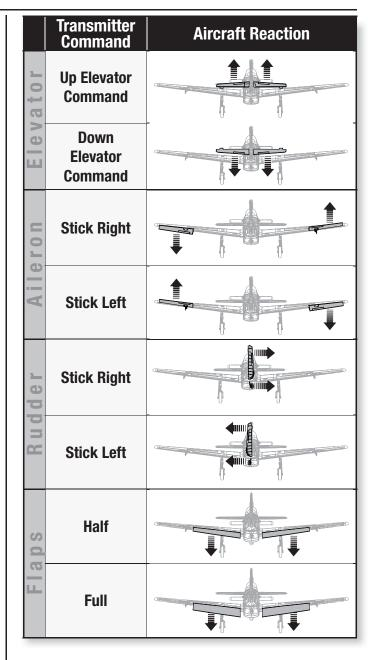
This test ensures that the AS3X control system is functioning properly. Assemble the aircraft and bind your transmitter to the receiver before performing this test.
