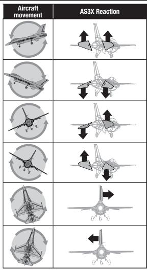
Arrows indicate the direction of the trailing edge of the control surface.
