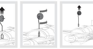
Make sure to reinstall the nose gear angled forward as shown.
