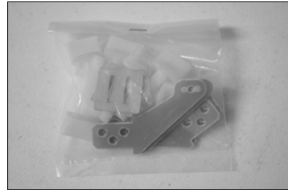
Aileron and Elevator Control Horns, Plates and Nylon Wing Bolts
