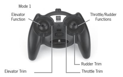
Note: Before each flight you should ALWAYS turn the transmitter on before connecting the flight battery to the receiver unit. After each flight, be sure that you always disconnect the flight battery from the receiver unit before powering the transmitter off.
