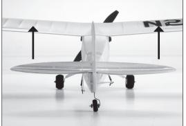
Move the rudder stick left and right to check yaw control. When the stick is pushed to the right, the rudder should also move to the right.
