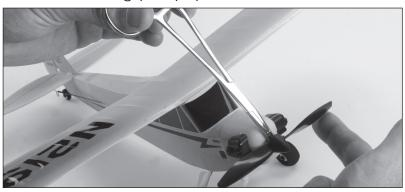
2. Spin the propeller counterclockwise (if viewed from the front) to remove the old propeller.
