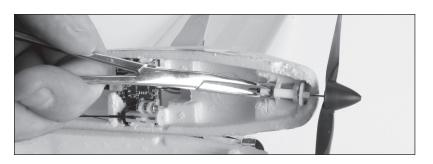
3. While holding the nylon nut, rotate the spur gear in a clockwise direction. The prop shaft will thread out of the nut.
