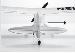
With the rudder stick pushed to the left, the rudder should move to the left.
