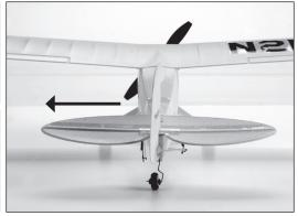
If at any time during the test the controls respond in the opposite direction, it may be necessary to reverse/change the direction of operation of the flight controls. Follow the Reversing Flight Controls section to change the direction of the various flight controls.
