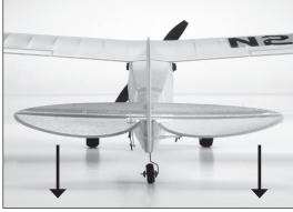
When the elevator stick is moved aft, the elevator should move up.
