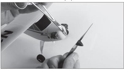
3. Thread the new 100mm x 60mm prop and spinner clockwise onto the gearbox shaft.
