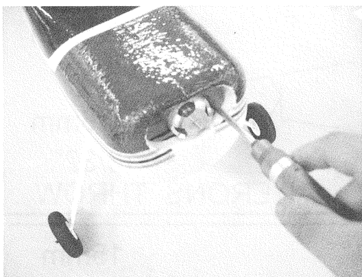
使用2.6 x 10 mm木工螺絲安裝馬達。 Use 2.6 x 10mm tapping screw to secure the motor in place.
