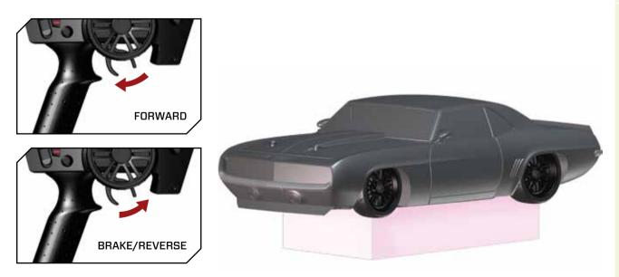
Perform a control test with the vehicle wheels off the ground. If the wheels rotate after the vehicle is powered ON, adjust the "TH. Trim" knob until they stop. To make the wheels move forward, pull the trigger. To reverse them, wait for the wheels to stop, then push the trigger. When moving forward, the wheels should maintain a straight line without any steering wheel input. If not, adjust the "ST. Trim" knob so the wheels maintain a straight line without having to turn the steering wheel.
