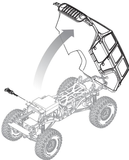
**INSTALLARE LA BATTERIA DEL VEICOLO**
