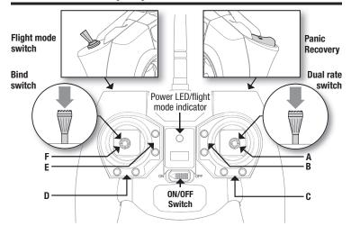
When pressed down, trim buttons make a sound that increases or decreases in pitch at each pressing. The middle or neutral trim position is heard as a middle tone in the pitch range of the sounds. The end of the control range is sounded by a series of beeps.
