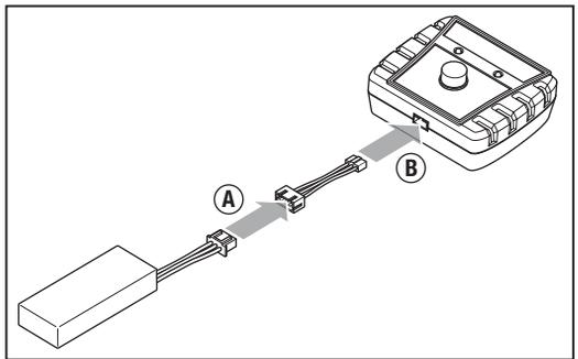
Charging a fully discharged (not over-discharged) 800mAh battery takes approximately 60 minutes.
