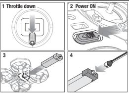
CAUTION: Always disconnect the Li-Po battery from the aircraft when not flying to avoid over-discharging the battery. Batteries discharged to a voltage lower than the lowest approved voltage may become damaged, resulting in loss of performance and potential fire when the batteries are charged.
