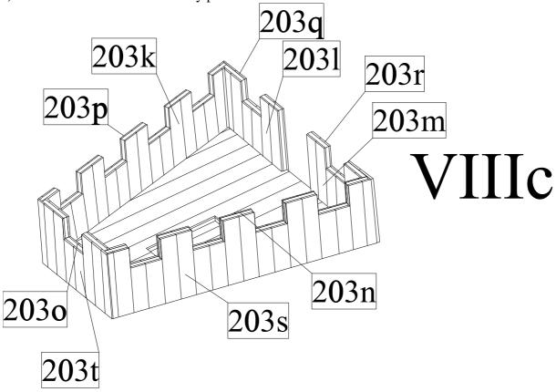
d) Border a deck of the fore castle by strips 120 and then glue to the walls also inner and outer reinforcement beams 121 and 122. The fore castle is in 1:1 scale shown in the plan 3H.
