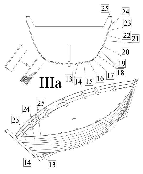
b) By a sharp knife cut out parts of the frames which exceed the deck. Then by a sand paper sand remains of material.
