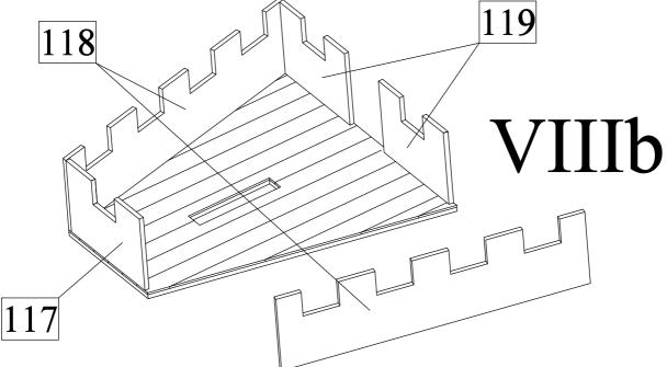
c) Plank the side walls 117-119 by parts 203.
