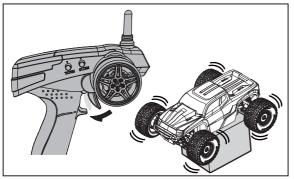
2. Connect the battery to the Electronic Speed Control (ESC) / Receiver unit and power on the vehicle.
