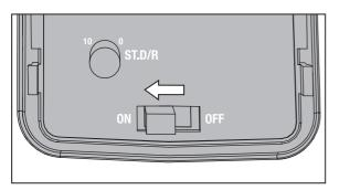
3. Do a test of the transmitter's control of the vehicle with the vehicle's wheels off the ground.
