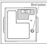
You must rebind when binding the receiver to a different transmitter.
