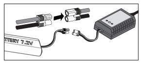
The vehicle battery charger produces 2000 milliAmps (2 Amps) per hour. Divide the mAh capacity on the label of a battery by 2000 to know how long battery charging will require. For example, an 1800mAh battery requires 0.9 hours (54 minutes) to charge.
