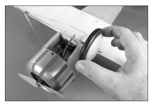
OO 5. Slide the wheel retainer onto the landing gear wire. Use a drop of foam-safe CA on the side away from the wheel to secure the retainer. Make sure not to get CA on the wheel or axle, preventing the wheel from rotating.
