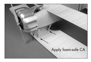
O 5. Position the outer strut in the slots in the top and bottom wing. The strut will angle back from the top wing down to the bottom wing. Use foam-safe CA to glue the wing strut to the underside of the top wing.
