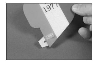
O 8. Apply a few drops of foam-safe CA to the joint between the tab on the control horn and control horn backplate to prevent it from coming loose.
