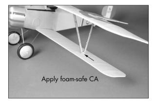
7. Repeat Steps 5 and 6 to install the remaining outer strut.
