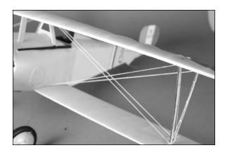
O 17. Use tape or weights to keep the wheels secure on your work surface while setting the line tension and position.
