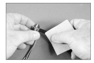
5. Mount the speed control using two-sided tape to the front of the fuselage as shown below. Route the servo lead back to the receiver and plug it into the throttle port of the receiver. Use a tie wrap (not included) to keep the wires from interfering with the operation of the motor.
