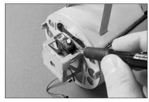
3. Use a pin drill and 1/16-inch (1.5mm) drill bit to drill the holes for the two servo mounting screws.
