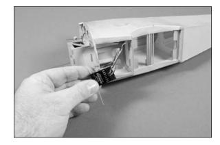
O 17. Use two-sided tape to secure the receiver in the fuselage as shown.
