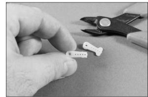
OO 8. Use a pin drill and 1/16-inch (1.5mm) drill bit to enlarge the outermost hole in the servo arm.
