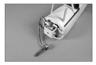
7. Slide the carbon tube into the hole in the fuselage. There are two hoes that will provide the proper alignment of the motor.
