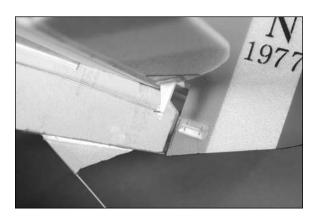
2. Slide a micro pushrod keeper onto the wire extending through the control horn.
