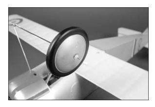
O 6. Install the remaining wheel and secure it following the procedure described in Steps 4 and 5.
