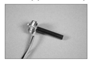
4. Use medium grit sandpaper to roughen the outside of the carbon tube so the CA used to glue it in the fuselage has a surface to attach to.
