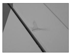
O 6. Attach the micro control connector to the servo arms. Be sure to use the included retainer to secure the micro control connector to the servo arm.
