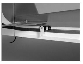
Q 2. Use a hobby knife to enlarge the center hole in one of the remaining control horns. Attach the 3" (75mm) pushrod wire to the control horn. • 3. Attach the micro control horn to the elevator using the control horn backplate and 6-minute epoxy.
