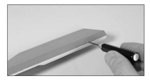
• 2. Slide four hinges into the slits in the aileron. Center the slot in the hinge with the hole drilled in Step 1. Place a T-pin in each hinge to prevent it from being pushed into the wing when installing the aileron.
