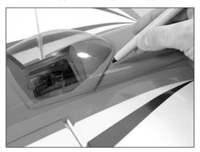
• 3. Lightly sand the inside edge of the canopy where it contacts the hatch. Also sand the hatch inside the line drawn in the last step.
