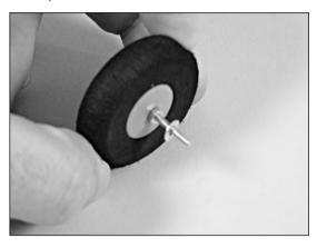
O 2. Fit the assembly from Step 1 into the wheel pant. Use a 2mm washer and nut to attach the wheel to the lower hole on the landing gear.
