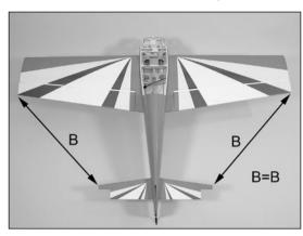
• 3. View the airframe from the rear and make sure the wing and stab are parallel. If not, lightly sand the stab saddle until they are.
