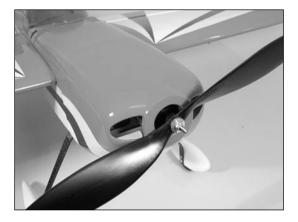
**Note**: It is very important that you check to be sure the propeller is balanced before installing onto the shaft. An unbalanced propeller may strip the gear. When installing the propeller, please do not over-tighten the 3mm locknut. The use of the locknut will prevent the propeller from coming loose.
