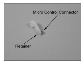
○ 7. Turn on the radio system and center the aileron trim and stick. Make sure the aileron servo is operating properly using the transmitter. Slide the pushrod wire through the micro connector. Install the servo arm 90-degrees to the servo. Center the aileron, and secure the position of the wire using the 2mm x 4mm screw and a Phillips screwdriver.
