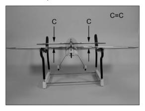
4. Double-check the adjustments from Steps 1 through 3. Use a felt-tipped pen to trace the outline of the fuselage onto the top and bottom of the stabilizer.
