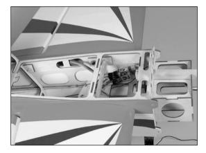
**Note**: Do not cut the receiver antenna, as this will greatly reduce the range of the radio system.
