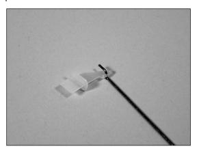
O 5. Use 6-minute epoxy to attach the control horn to the aileron.
