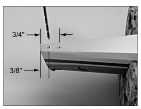
O 5. Glue the tail skid into position using Medium CA.
