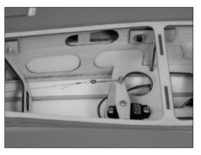
• 12. The cables will cross inside the fuselage to get the proper geometry for the rudder to operate correctly.
