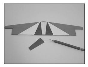
O 6. Hinge the elevator and stabilizer, using the same process as described in Aileron Hinging. Use 4 hinges for this process.
