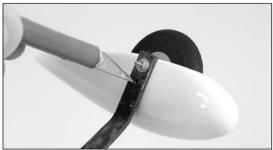
O 8. Secure the location of the wheel pants using 2mm x 6mm wood screws and a small Phillips screwdriver.
