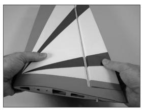
O 5. Work the aileron up and down several times to work in the hinges and check for proper movement.
