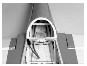
O 13. Remove the tape from the control surface. Install the second cable following Steps 9 through 11. Tension the cables lightly using the cable connectors to pull the surface into neutral.
