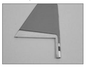
3. Position the fin back onto the fuselage. Use a square to check the alignment between the fin and stabilizer. Lightly sand the bottom of the fin until the alignment is correct.
