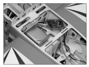
**Hint**: You may use a piece of hook and loop strapping around the battery to help secure it in position.
