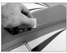
• 4. Glue the canopy to the hatch using canopy glue. Tape the canopy into position until the glue cures.
