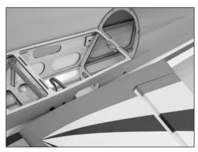
○ 3. Slide the remaining wing panel into position. Secure the panels using 4-40 x 1/2" socket head screws with #4 washers (silver) using a 3/32" hex wrench.
