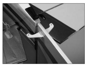
O 6. Install the grommets and brass eyelets in the rudder servo. Mount the rudder servo using the hardware provided with the servo.
