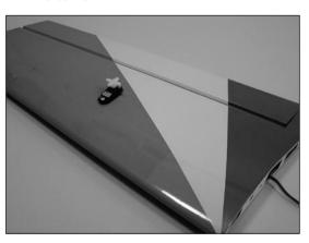
• 4. Use a hobby knife to enlarge the center hole in the control horn to fit the 3  $^3/_8$ " (85 mm) long aileron pushrod wire.
