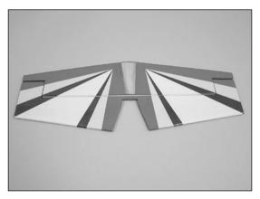
7. Slide the stab and elevator back into position. Again, check the alignment and make sure everything lines up. Wick Thin CA into the joint between the fuselage and stabilizer. Make sure to glue both top and bottom. Do not use accelerator—allow the CA to wick in as far as possible, providing the best bond. Place the filler plug in place behind the elevator, but do not glue at this time.
