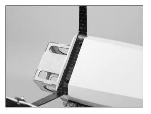
7. Place the fuselage on its wheels and position the wheel pants parallel to the work surface. Drill a hole through the landing gear into each wheel pant using a hobby knife.
