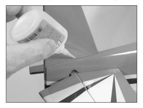
5. Attach the rudder using three CA hinges. Use the technique as described in Aileron Hinging for this procedure. Use thin Ca to glue the filler plug at the rear of the fuselage.
