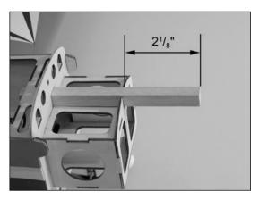
• 4. Slide the gearbox into position on the motor support stick. Use a hobby knife to make a hole in the gearbox and into the motor stick. Secure the gearbox to the motor stick using a 2mm x 8mm sheet metal screw.
