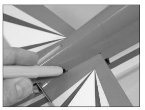
O 5. Use a sharp hobby knife to cut the covering slightly inside the lines drawn. Be very careful not to cut into the underlying wood, as this will weaken the stab and cause it to fail in flight.
