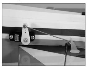
**Note**: An optional rudder servo location has been provided at the rear of the fuselage if using heavier motors and you choose not to use the pull-pull system. The installation procedure is identical to the elevator servo installation, except the covering must be removed from the fuselage first.
