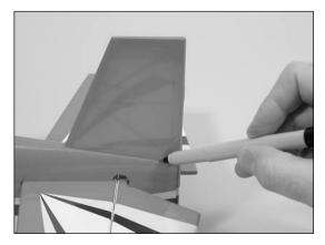
• 2. Remove the covering from the bottom of the fin using the same technique used for the stabilizer.
