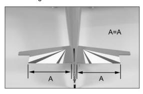
2. Measure from the stab tip to the wing tip. Adjust the stab until the measurements are equal.
