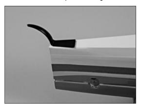
• 6. Attach the landing gear using a 3/32" hex wrench, two 4-40 x 1/2" socket head screws and two #4 washers (black).
