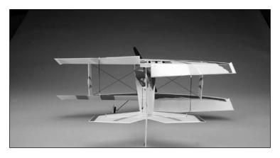
With the aileron stick pushed right, the right aileron should move up and the left aileron should move down.
