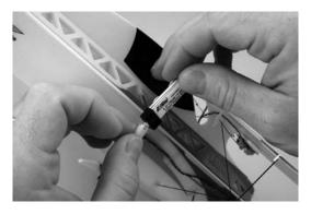
2. Mount the battery in the airplane by placing it onto the bottom of the horizontal fuselage on the right-hand side where the hook and loop strip is located. The plug will face toward the rear of the airplane.
