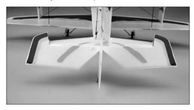
When the elevator stick is moved aft the elevator should move up.
