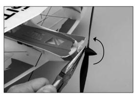
2. Install the new prop in the same manner twisting it back onto the shaft in a clockwise manner. The prop is fully installed when all of the threads on the shaft are not visible outside of the prop.
