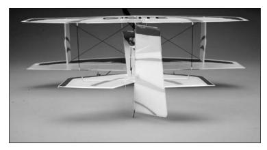
With the rudder stick pushed to the left, the rudder should move to the left.
