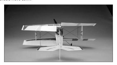
Move the rudder stick left and right to check yaw control. When the stick is pushed to the right the rudder should also move to the right.
