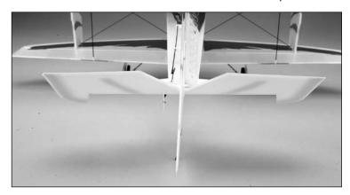
Move the aileron stick left and right to check aileron roll control. When the stick is pushed to the left, the left aileron should move up and the right aileron should move down.
