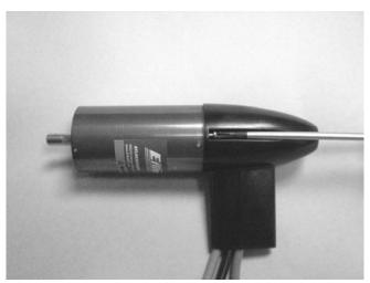
1. Slide the motor wires into the center body fairing as shown. 2. Connect the center body fairing to the back of the motor using the two 2mm x 5mm screws provided. Note: You may want to trial fit the center body fairing so you can make sure the wires are accessible to plug into the ESC when the motor is attached to the fan unit. You may have to re-position the fairing before attaching to the motor.
