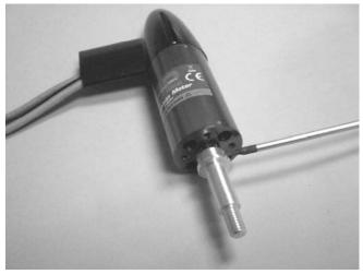
3. Slide the threaded shaft onto the motor shaft and tighten both set screws. Use removable blue thread lock.
