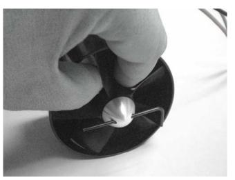
6. Screw the spinner onto the threaded shaft and tighten while holding the spinner in place making sure it is secure. Use an L-wrench or something similar to help tighten the spinner.
