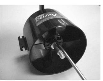
4. Attach the motor to the fan unit using the two 3mm x 5mm screws provided.
