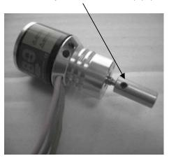
Screws used to Mount EDF to Motor (4)
