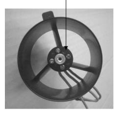
Screw Attaching Rotor
