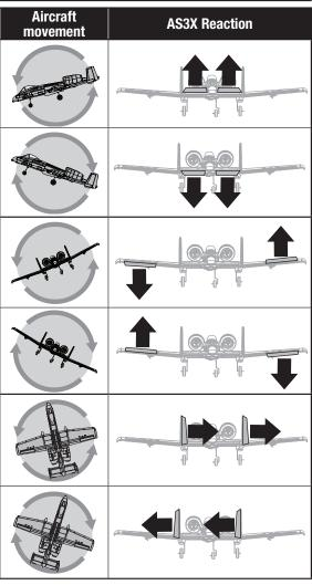
Arrows indicate the direction of the trailing edge of the control surface.
