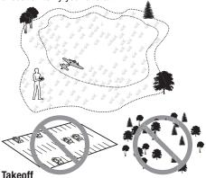
Place the aircraft in position for takeoff (facing into the wind if flying outdoors). Set dual rates to low position and gradually increase the throttle to ¾ to full and steer with the rudder. Pull back gently on the elevator and climb to check trim. Once the trim is adjusted, begin exploring the flight envelope of the aircraft.
