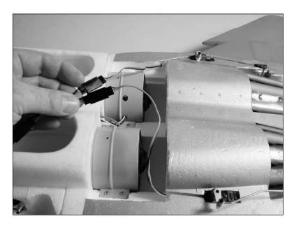
13. Slide the servo extension into the opening between the fan tunnels at this time.
