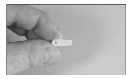
9. Use a hobby knife to enlarge the outer hole of a servo arm. Install the pushrod connector and secure it using the nylon nut supplied with your model.
