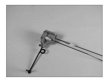
O 15. Use four 2mm x 8mm sheet metal screws and a #1 Phillips screwdriver to secure the nose gear. Note that the spring for the gear faces to the front of the fuselage. Slide the wheel onto the gear. Press a spring washer onto the wire to secure the wheel.
