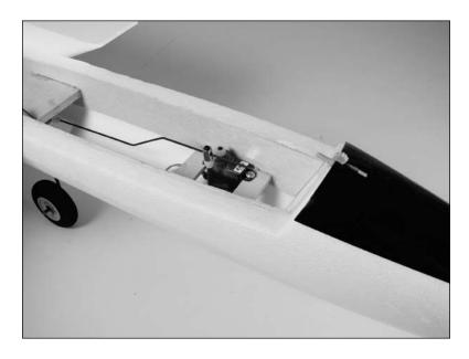
**Note**: You will need to bend the nose gear pushrod slightly to achieve the correct alignment between the servo and nose gear.
