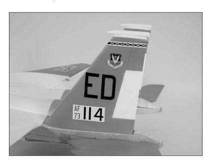
Check the alignment between the right and left fins.
