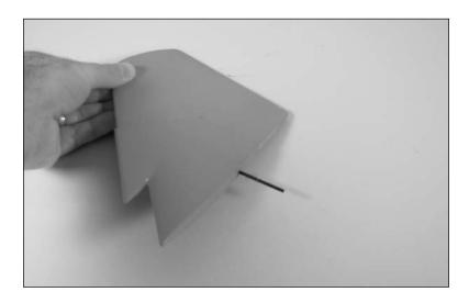
3. Slide the appropriate stabilator into the bushing in the fuselage. As you slide the stabilator in position, slide it into one of the control ball ends.
