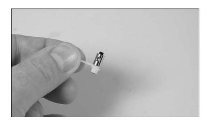
OO 6. Snap the ball link on the 145mm pushrod onto the stabilizer control ball end.
