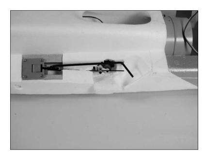
OOO11. Use side cutters to cut the excess wire that may interfere with the operation of the retract.
