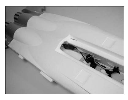
10. Repeat Steps 1 through 9 to install the remaining fan assembly in the fuselage.
