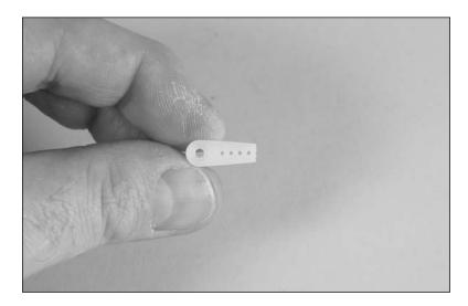
O 18. Use a hobby knife to enlarge the outer hole of a servo arm. Install the pushrod connector and secure it using the nylon nut supplied with your model.
