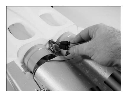
O 14. Use clear tape to secure the elevator servo leads to the fan shroud. This will prevent the wiring from interfering with the operation of the fans.
