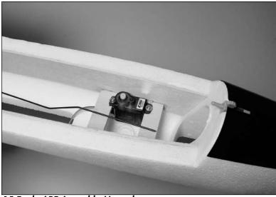
8. Use side cutters to remove the outer hole from the servo arm. This is done in case you will be installing retracts later in the life of your model.
