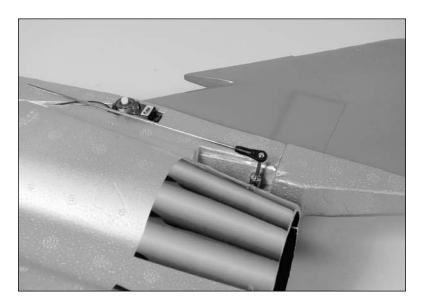
7. Slide the pushrod connector onto the pushrod wire. After centering the elevator servo using the radio, install the servo arm on the elevator servo. Make a small bend in the pushrod to ensure the pushrod is straight and in line with the control arm.
