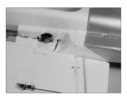
2. Position the wing so it is parallel to your work surface when viewed from the front of the aircraft. Makle sure the fuselage is parallel to the work surface as well. Use 6-minute epoxy to glue one wing panel to the fuselage. Use painter's tape to keep the wing tight against the fuselage while the epoxy cures.
