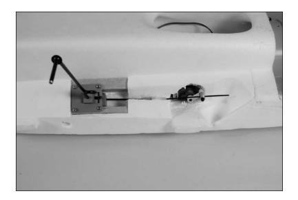
20010. Use the radio to move the servo to the "up" position, then move the retract linkage. Check the line made on the wire to see if it is in the same location as it was in the "down" position. If not, use the end point adjustment of the radio to fine-tune the servo so the line on the pushrod is in the same position when the servo is in both the "up" and "down" positions. Once the servo has been adjusted, use a 1.5mm hex wrench to tighten the setscrew and secure the pushrod.
