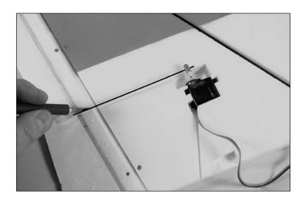
5. Use 6-minute epoxy to glue the control horn in the aileron as shown.
