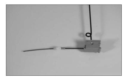
**Important**: You may need to shave the plastic retract connector on the retract actuator arm to ensure the clevis pin snaps closed.
