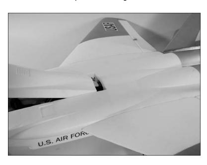
2. Slide the canopy catch forward and press the canopy hatch down. Release the catch into position to secure the canopy.
