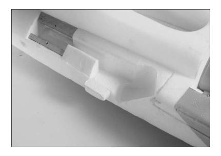
4. Carefully cut a hole in the side of the fuselage to install the main gear retract servo. Make sure to allow for clearance of the servo arm.
