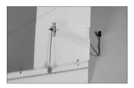
O 8. Repeat Steps 1 through 7 to install the remaining aileron servo and linkage.
