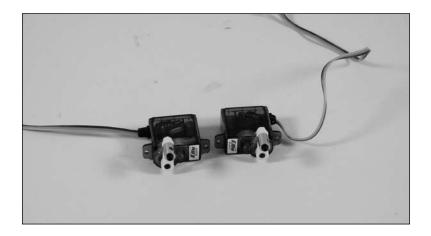
3. Use 6-minute epoxy to glue the aileron servo into the wing. Note that the servo arm faces toward the aileron. Press the servo lead into the channel in the wing as shown.
