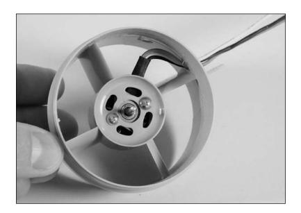
**Note**: You might have to grind a small hole in the shroud to accommodate your motor leads.
