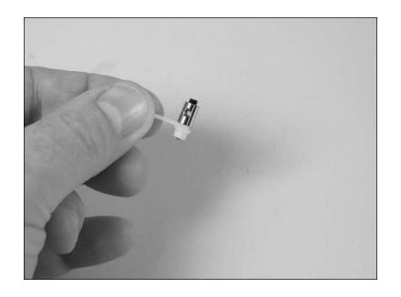
O 10. Slide the pushrod connector onto the pushrod wire. After centering the steering servo using the radio, install the servo arm on the steering servo. Center the nose wheel and secure the pushrod wire using the setscrew and 1.5mm hex wrench.
