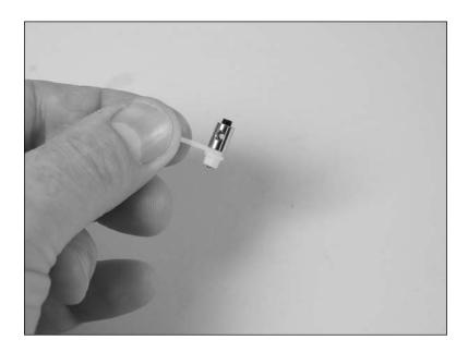
2. Install the servo arm on the aileron servos. Make sure to center the aileron servos using the radio system before installing the servo arms.
