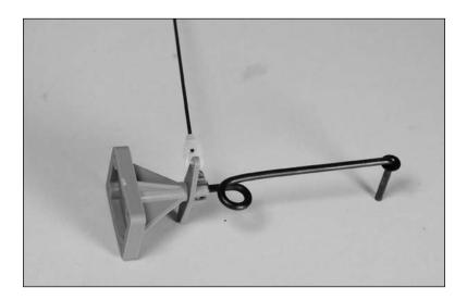
5. Use four 2mm x 8mm sheet metal screws and a #1 Phillips screwdriver to secure the nose gear. Note that the spring for the gear faces to the aft of the fuselage.
