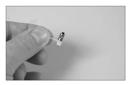
19. Slide the pushrod connector onto the pushrod wire. After centering the steering servo using the radio, install the servo arm on the steering servo. Center the nose wheel and secure the pushrod wire using the setscrew and 1.5mm hex wrench. Using a Y-harness, plug the nose gear retract servo into the gear channel. Repeat Steps 9, 10 and 11 to adjust the nose gear retract servo. You should find the nose retract servo will be very similar in endpoints to one of the main retract servos.
