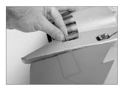
4. Once the stabilator is positioned, rotate it so the setscrew can be accessed. After applying a drop of threadlock on the setscrew, use a 1.5mm hex wrench to tighten the setscrew onto the flat of the control rod.
