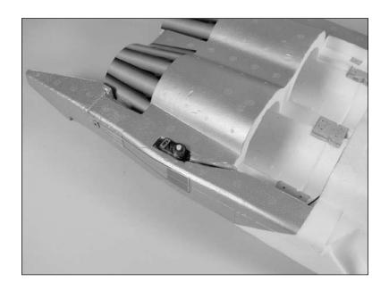
2. Locate the stabilator and look at the rod of the stabilizer. You will note that one side of the control rod has a flat area ground onto the rod. This will face to the top of the fuselage when the stabilator is installed.
