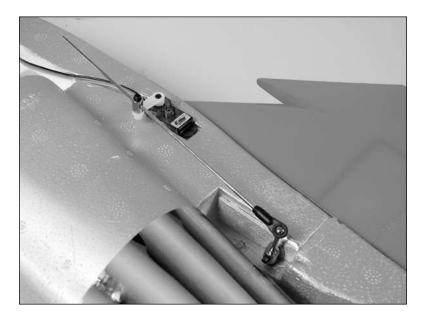
8. With the radio system on, center the stabilator using the guide on the side of the fuselage. Tighten the setscrew to secure the pushrod wire to the elevator servo. Make sure to use threadlock on the setscrew to prevent it from vibrating loose.
