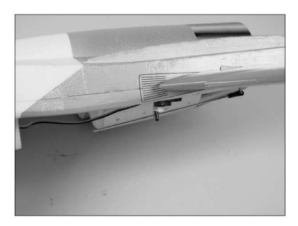
9. Repeat Steps 1 through 8 to install the remaining elevator servo. Make note that the pushrod is bent slightly and the servo arms of both elevator servos face the same direction. This will make both stabilators operate in the same direction without the need to use mixing at the radio.
