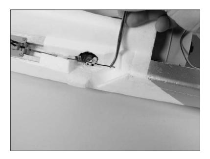
12. Slide the wheel onto the gear. Press a spring washer onto the wire to secure the wheel.
