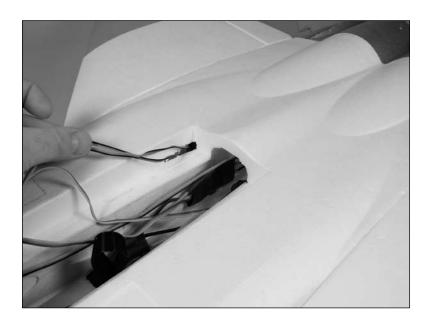
2. Secure the receiver on the top side of the same plywood plate the nose gear is attached to, using hook and loop tape. Plug the servo leads for the elevators, ailerons, retracts, nose gear steering and speed controls into the receiver. Use a Y-harness between each of the speed controls, between the aileron servo extensions and one of the main and nose gear retracts.
