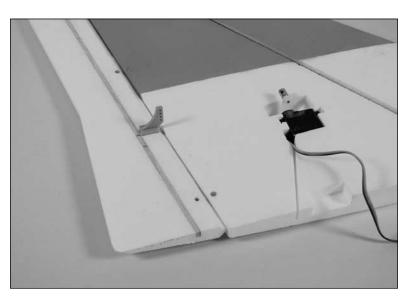
6. Connect the clevis to the control horn. With the aileron and aileron servo centered, tighten the setscrew in to connector with a 1.5mm hex wrench to secure the pushrod wire.
