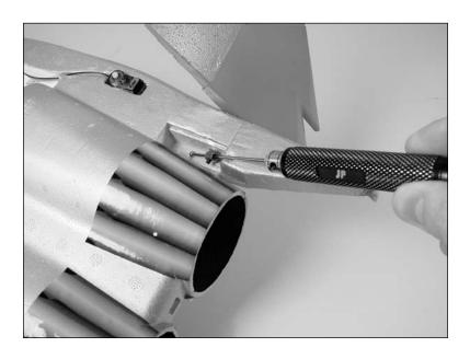
5. Use a hobby knife to enlarge the outer hole of a servo arm. Install the pushrod connector and secure it, using the nylon nut supplied with your model.
