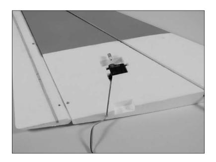
4. Slide a 75mm pushrod wire into the hole in the connector. Use a hobby knife to cut a 2mm wide slot in the aileron near the hinge line using the wire as a guide. Keep the wire perpendicular to the servo while cutting the slot.
