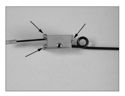
7. Carefully remove the actuator arm and move it so the actuator is on the same side as the gear strut. Install the screws and check that the retract moves smoothly without any binding.
