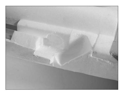
5. Fit the retract servo into the fuselage. It will extend into the intake as shown. Make sure the servo fits in far enough so the hole in the connector aligns with the center line of the slot for the retract gear wire. Use 6-minute epoxy to glue the servo in position.
