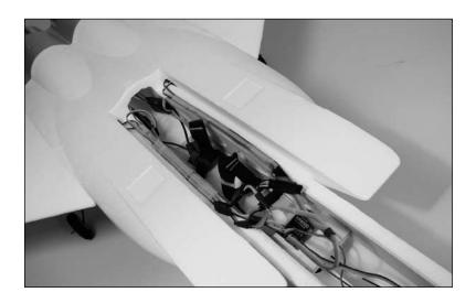
3. Use clear tape to secure the servo leads neatly inside the battery compartment. Doing so will make the installation and removal of the batteries much easier.
