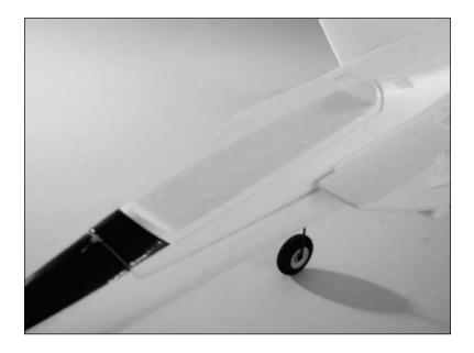
3. Use canopy glue to glue the canopy to the canopy hatch. Use painter's tape to keep the canopy in position until the glue fully cures.
