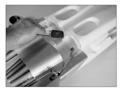
8. Secure the fan to the fuselage using four 2mm x 8mm sheet metal screws and a #1 Phillips screwdriver.
