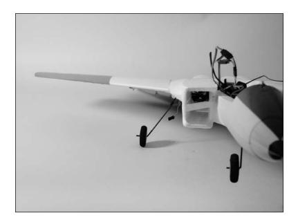
3. Repeat Steps 1 and 2 to attach the remaining wing panel to the fuselage. Make sure the alignment of the second wing panel matches that of the first panel so the aircraft has an equal amount of dihedral for both right and left panels. If the dihedral does not match, it may require a lot of trim to correct and will not provide the best flight performance.
