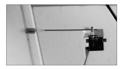
7. Use the supplied tape to cover the aileron servo and wire as shown. You may now cover the carbon spar with the white and orange tape.
