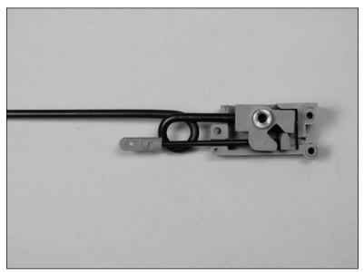
8. Attach the clevis from a 127mm pushrod to the retract actuator. Slide the tubing over the clevis to secure the clevis and prevent it from opening accidentally.
