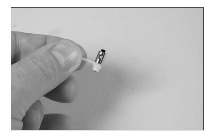
2. Install the servo arm on the main gear retract servo. The servos shown are centered. You will want an equal amount of throw in both directions from this center position when operating the retract servos.
