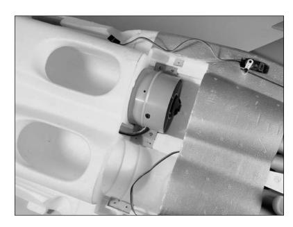
9. Secure the speed control to the side of the fuselage using hook and loop tape.
