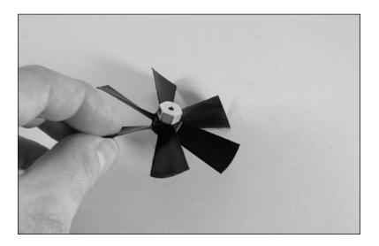
2. Use the impeller nut to secure the impeller shaft to the impeller. Do not tighten at this time.
