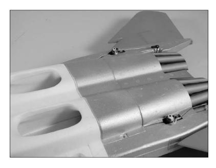
**Note**: You might have to remove a small amount of foam from the inside area of the Power Hatch to allow the hatch to fit down nice and tight. This is due to the wires from the stab servos running through this area.
