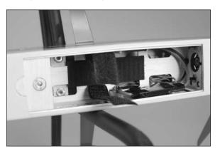
8. Apply the matching hook and loop tape from step 5 to the bottom of the battery. This will keep the battery from moving forward or aft in the fuselage. Use the hook and loop strap to secure the battery to the battery tray.
