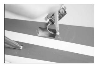
3. Apply 1-2 drops of thin CA in each of the holes to harden the surrounding wood. This will harden the threads so the screws do not easily strip the surrounding wood.
