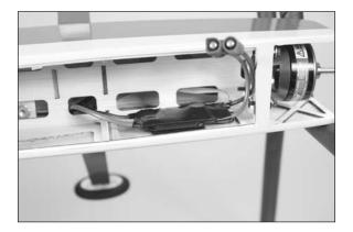
6. Route the lead from the speed control through the fuselage and plug it into the throttle channel of the receiver. Cut a small section of hook and loop tape to secure the receiver in the fuselage. Set the receiver back from the wing tube so the aileron servo leads can be inserted into the fuselage without interference from the receiver.
