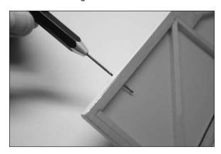
2. Place a T-pin in the center of each of the five hinges. This will center the hinges equally in the aileron and wing when they are installed.
