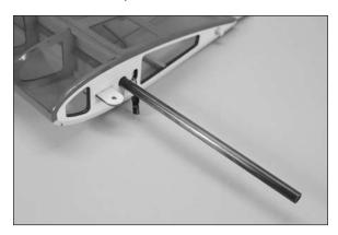
Slide the tube into the socket in the fuselage.
