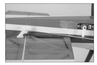
9. Slide the control horn backplate over the end of the control horn from the opposite side of the control surface. Snap the backplate so the horn is held tight against the control surface. Apply 2–3 drops of thin CA to the backplate where it contacts the control horn to keep it from accidentally coming loose in flight.
