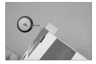
10. Use a pin vise and 1/16-inch (1.5mm) drill bit to drill a hole in the center of each hinge slot to create a tunnel for the CA to wick into. This will allow the CA to penetrate the hinge, creating a better bond between the hinge and surrounding wood. Prepare the rudder and vertical fin at this time.
