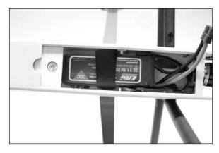
9. Turn on the transmitter. Connect the battery to the power lead of the speed control. Check the rotation of the motor to make sure it rotates counterclockwise when viewed from the front of the fuselage. If not, swap any two of the motor leads to correct the direction of rotation.
