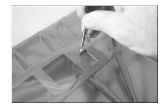
2. Apply 1–2 drops of thin CA in each of the holes to harden the surrounding wood. This will prevent the screws from stripping surrounding wood.
