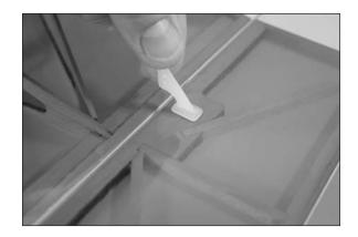
2. Slide the control horn backplate over the end of the control horn from the opposite side of the control surface. Snap the backplate so the horn is held tight against the control surface. Apply 2–3 drops of thin CA to the top and bottom of the horn backplate to keep it from accidentally coming loose in flight.
