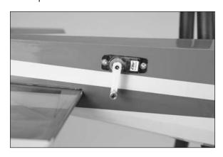
7. Pass the Z-bend in the elevator pushrod through the center hole (inner hole for the rudder) of the control horn.
