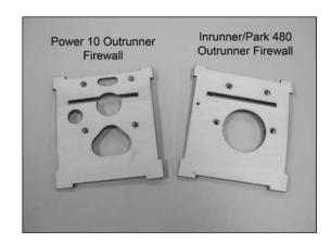
Q 2. Attach the firewall to the sub-firewall structure on the front of the fuselage nose at this time using 6-minute epoxy or thick CA. Epoxy is best for this application. Make sure all joints are secure when finished so the firewall does not detach from the sub-firewall.
