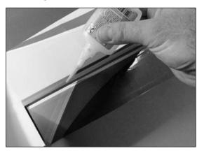
Q 4. Firmly grasp the wing and aileron and gently pull on the aileron to ensure the hinges are secure and cannot be pulled apart. Use caution when gripping the wing and aileron to avoid crushing the structure.
