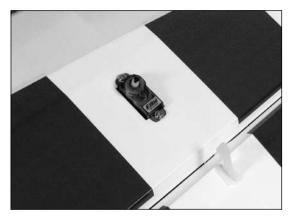
○ 4. Attach the 3" (75mm) pushrod to the control horn. Start the wire from the wing tip side of the control horn.
