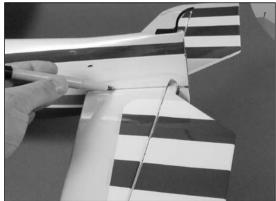
7. Use a sharp hobby knife to cut the covering slightly inside the lines drawn. Be very careful not to cut into the underlying wood, as this will weaken the stab and cause it to fail in flight.
