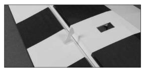
○ 2. Attach a 6" servo extension to the aileron servo. Secure the extension using string or a commercially available clip.
