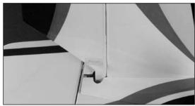
3. Install the micro control connector onto the elevator servo arm. Pass the elevator pushrod wire through the connector. With the radio on and elevator trim centered, center the elevator. Secure the elevator pushrod wire using the 2mm x 4mm screw and a small Phillips screwdriver.
