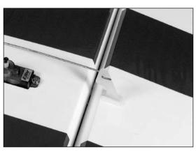
O 5. Attach the micro control connector to a long 3D servo arm. Be sure to use the included retainer to secure the micro control connector to the servo arm. Remove the remaining unused part of the servo arm.
