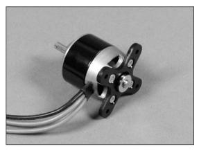
Q 2. Using four 4-40 x 43mm socket head screws and washers and outrunner offset spacers, attach the motor with X-mount to the blind nuts on the firewall The offset spacers have already been sized correctly so you have proper clearance when the cowling is installed later.
