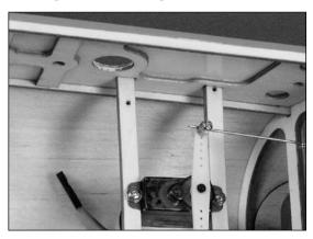
O 8. The cables will cross inside the fuselage to get the proper geometry for the rudder to operate correctly.
