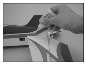
9. Install the four carbon rods between the fuselage and stabilizer as shown. Glue the rods to the stabilizer and fuselage using 6-minute epoxy.
