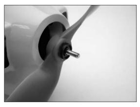
**Note**: Two spacers have been provided that are placed between the propeller and spinner backplate. Use the thin spacer for low-pitch propellers, the thick spacer for high-pitch propellers. This will prevent the blades of the propeller from contacting the spinner backplate.
