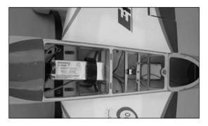
*Hint*: It is recommended you may use a piece of hook and loop strapping around the battery to help secure it in position.
