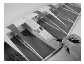
**Important**: Do not cut into the underlying wood. This will weaken the structure and could cause failure in flight. As an option, you can use a soldering iron or hot knife with light pressure to carefully melt the covering and avoid the potential of cutting into the wood. 4. Slide the wing back into position in the fuselage. Check to make sure the wing is perpendicular (90°) to the fuselage as shown. Lightly sand the opening in the fuselage if necessary to make any adjustments.
