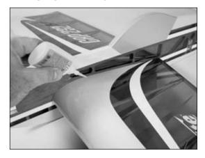
**Note**: Avoid using a CA accelerator to allow the CA to wick well into the wood of the fuselage and wing. This will provide the best bond between the two items.
