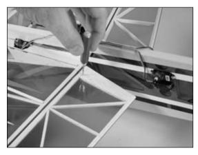
○ 7. Slide the control horn into the holes from the bottom of the aileron. Apply a few drops of thin CA to the posts from the top of the aileron. Slide the control horn backplate into position, making sure the horn is solidly secured. Apply a couple drops of thin CA where the posts protrude through the backplate.
