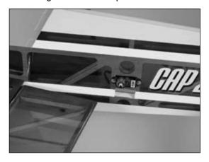
○ 3. The rudder servo is installed in the lower hole using the hardware provided with your servo. Pre-drill the holes for the servo mounting screws using a drill and 1/16" (1.5mm) drill bit. The output for the rudder servo will be opposite the elevator servo facing the front of the plane.
