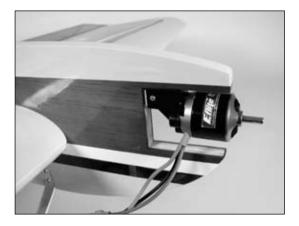
**Note**: Check that your motor has right thrust. The motor will be angled towards the right when viewed from the top of the aircraft as shown.
