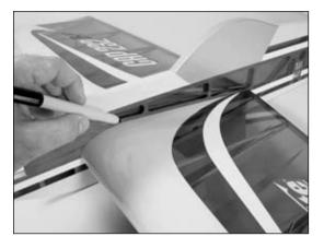
○ 3. Remove the wing and use a hobby knife with a sharp #11 blade to remove the covering from the wing 1/16" (1.5mm) inside the lines drawn.
