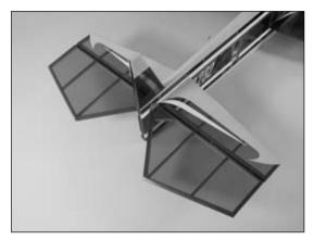
• 6. Hinging the rudder follows the same procedure as the elevators, except you don't have to worry about the elevator joiner. Use three CA hinges when attaching the rudder to the fin/fuselage.
