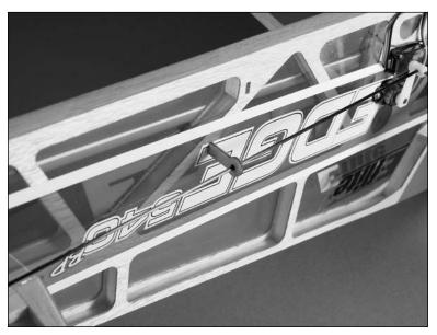
O 15. The last linkage to install is for operating the rudder. The long 13-inch (330mm) carbon pushrod is used for the rudder. Follow the same procedure as the elevator pushrod, including the installation of the pushrod guide.
