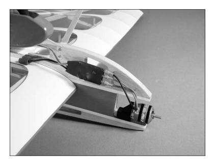
O 6.Attach the battery to the side of the fuselage using hook and loop tape. The exact position of the battery can be changed forward or back, depending on what is necessary to achieve the correct center of gravity. Turn on the radio system and plug the battery into the speed control. Use the throttle to check that the motor rotates counterclockwise when viewed from the front. If not, follow the directions included with your speed control to change the direction of the motor rotation.
