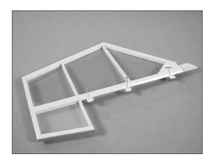
O 4. Slide the hinges and elevator into position on the stabilizer. Align the end of the elevator with the end of the stabilizer. Remove the T-pins to position the elevator as close to the stabilizer as possible while maintaining proper hinge gap for adequate throw. Saturate each hinge, top and bottom, with thin CA.
