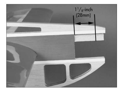
O 3.Use medium CA to glue the two motor offset shims to the sides of the motor stick. This is necessary to provide the correct thrust angle for the motor. Make sure the thin end on the left shim is towards the front, and the shim on the right has the thick end of the shim towards the front.
