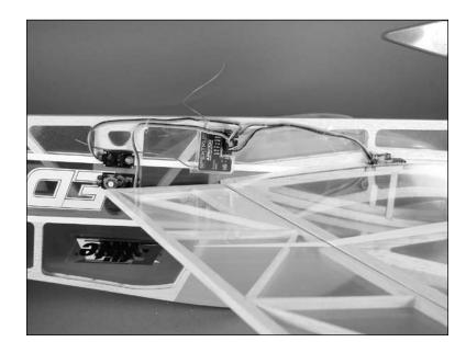
**Note**: Make sure all the wires are neatly taped to the fuselage to prevent them from getting entangled with the linkages.
