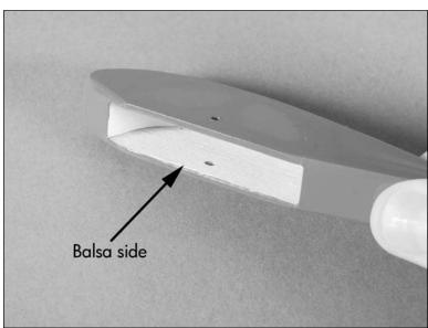
○ ○ 6. Slide the wheel into the wheel pant. The <sup>3</sup>/<sub>16</sub>-inch (5mm) offset on the spacer will be on the balsa side of the wheel pant. Pass the 4-40 x 1-inch socket head screw through the pant and into the spacer. Use pliers to hold the 4-40 nut inside the wheel pant on the plywood side and thread the screw into the nut.
