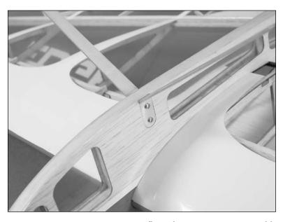
O 3. Locate one of the main wheels and the <sup>3</sup>/<sub>8</sub>-inch (10mm) spacer. Slide the spacer into the wheel.
