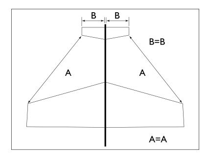
• 7. Check that the stabilizer and wing are parallel to each other. Lightly sand the opening in the fuselage to correct any alignment problems.
