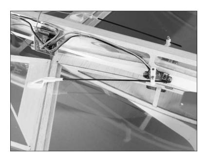
12.Slide the plywood pushrod support on the 11-inch (282mm) elevator linkage.
