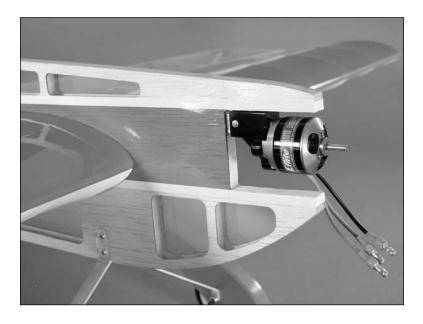
**Note**: You can also drill an extra screw in to the opposite side of the mount forward of the one shown to help reduce wear on the motor stick.
