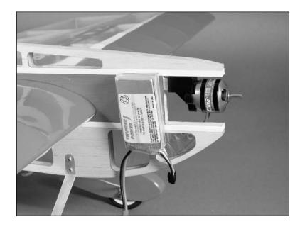
**Note**: Never check the motor rotation on the bench with the propeller installed. The plane could move and cause serious injury. Always check the motor without the propeller to avoid injury.
