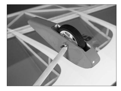
**Note**: The two 4-40 nuts will hold the wheel pant in position against the landing gear. You can apply a drop of thin CA between the luck nut and the gear to keep it from coming loose over time if necessary.
