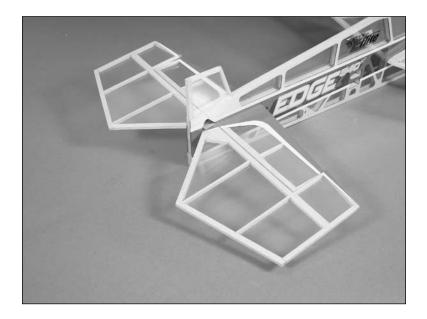
O 6.Hinging the rudder follows the same procedure as the elevators, except you don't have to worry about the elevator joiner. Use three CA hinges when attaching the rudder to the fin/fuselage.
