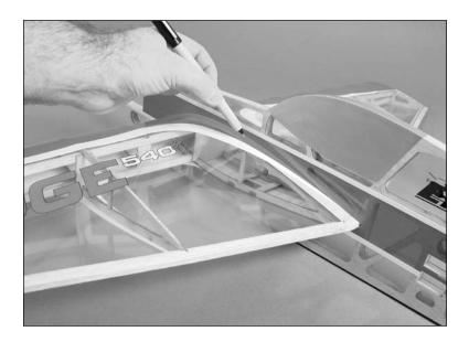
○ 3.Remove the wing and use a hobby knife with a sharp #11 blade to remove the covering from the wing <sup>1</sup>/<sub>16</sub>-inch (1.5mm) inside the lines drawn.
