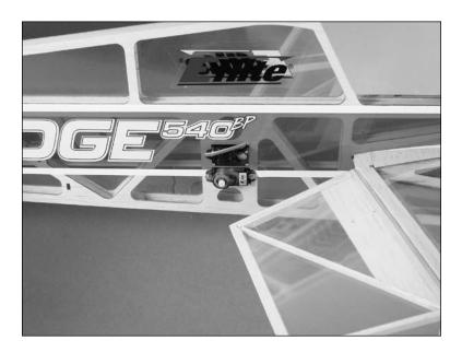
4. Secure the receiver to the fuselage under the wing using hook and loop tape. Route the antenna wires according to the manual provided with your radio system. Plug the servos into the appropriate positions in the receiver.
