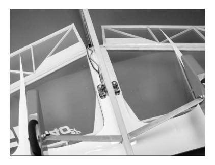
**Hint**: Pass both servo leads to the same side of the fuselage for a cleaner radio installation.
