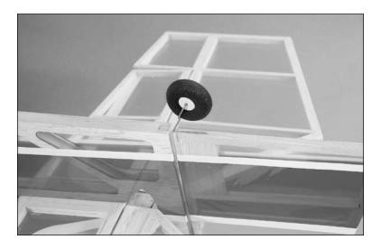
2. Attach the main gear to the fuselage using two 2mm x 15mm machine screws and the two 2mm nuts. Use a drop of thin CA or threadlock on the nuts to prevent them from vibrating loose.
