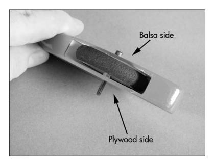
O 7. Slide the screw through the landing gear. Secure the wheel pant to the gear using a 4-40 lock nut. Tighten the 4-40 screw on to the locknut until the assembly is almost tight. At this point the wheel pant should still be able to rotate. Using pliers, hold the 4-40 nut inside the wheel pant and rotate the 4-40 socket head screw counterclockwise while positioning the wheel pant at the correct angle. This will tighten the wheel pant assembly between the two nuts.
