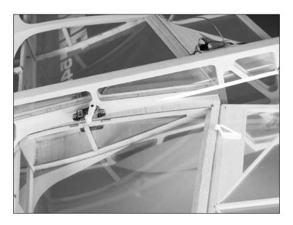
○ 9. Attach the 5<sup>3</sup>/<sub>8</sub>-inch (133mm) pushrod to the outer hole of the control horn.
