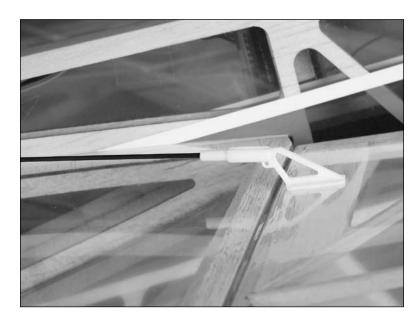
○ 10. With the radio system still on, physically center the aileron. Use the screw from the pushrod control connector to secure the pushrod to the connector.
