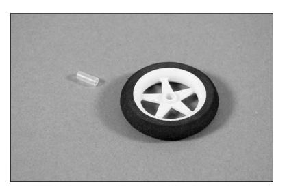
○ 4. Position the spacer in the wheel so it is offset to one side. The spacer will measure <sup>3</sup>/<sub>16</sub>-inch (5mm) on one side, <sup>1</sup>/<sub>16</sub>-inch (1.5mm) on the other. Use thin CA to glue the spacer on to the wheel once you have the correct offset.
