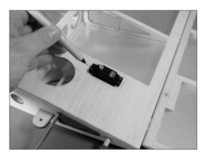
○ ○ 10. Use a pen drill and 1/16-inch (1.5mm) drill bit to drill the four locations for the servo mounting screws.
