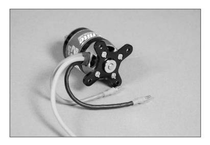
3. Use four 4-40 x 3/8-inch socket head screws to secure the motor to the firewall. The blind nuts installed behind the firewall can be moved to allow for the mounting of various sizes of motors.
