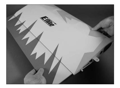
7. Flex the aileron through its range of motion a few times to break in the hinges.
