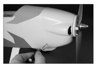
9. Secure the cowling using the four 2mm x 6mm sheet metal screws. There are two screws on each side of the cowl as shown. Complete the cowling installation by attaching the spinner cone using the two screws provided with the spinner.
