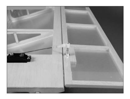
O O 16. Use a pushrod wire connector to secure the wire to the servo arm. Trim any excess wire using side cutters.
