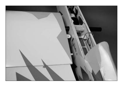
O O 3. Slide the remaining wing panel into position. Secure the panels using 4-40 x <sup>1</sup>/<sub>2</sub>-inch machine screws with #4 washers (silver) using a 3/32-inch hex wrench.
