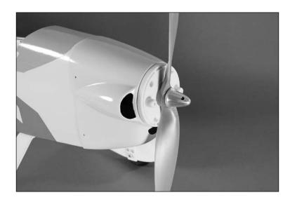
8. With the cowl aligned with the spinner, use a drill and 1/16-inch (1.5mm) drill bit to drill through the cowl and into the fuselage using the holes in the cowling.
