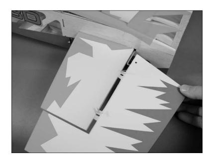
9. Rougher the joiner wire using medium grit sandpaper. Apply 30-minute epoxy to the joiner wire and in the hole in the elevator as well.
