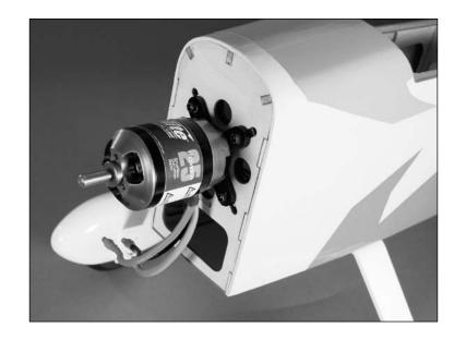
3. Plug the motor into the speed control. Use hook and loop tape to secure the speed control inside the fuselage out of the way of the battery.
