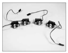
O 6. Use hot glue to install the aileron servos.
