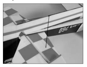
3. Check the alignment of the fin to the stabilizer. They should be perpendicular to each other. Check that the rods in the stabilizer are touching. Use foam-safe CA to glue the rods into position after checking alignment and that the rods are touching.
