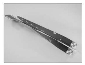
2. Locate the wing and slide it into the vertical fuselage underneath the horizontal fuselage. Use care not to damage either the vertical or horizontal fuselage pieces.
