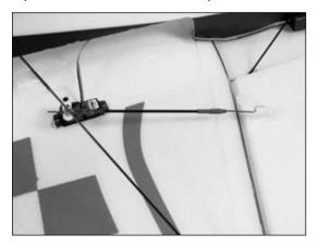
**Note**: Use the hole in the control horn closest to the aileron for the greatest amount of throw. Moving the pushrod outward, away from the aileron, will result in gradually decreasing the control throws.
