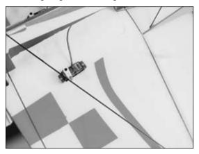
7. Install the rudder and elevator servos using hot glue. The output shafts of both servos face the front of the aircraft.
