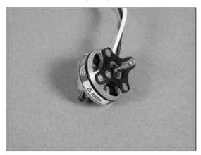
• 4. Attach the motor to the plywood mount using two #2 x 8mm wood screws or two #3 x 8mm wood screws.
