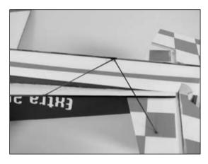
O 5. The next rod to install is the 4<sup>1</sup>/<sub>2</sub>" (113mm) rod from the rod in Step 4 to the bottom of the vertical fuselage.
