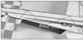
10. Install the receiver using hook and loop material. The exact position of the receiver may change, depending on how your aircraft balances.
