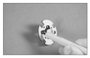
**Hint:** If the hole in your mount matches the diameter of the hole in the plywood mount, use a rolled-up piece of cardstock placed through the two holes to center the motor mount on the plywood mount.
