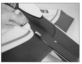
*Hint*: Use the holes for the aileron servos to aid in the alignment between the horizontal fuselage and wing.
