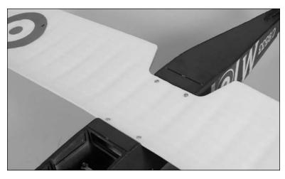
7. The installation of the top wing is identical to that of the bottom wing. Follow Steps 2 through 6 to attach the top wing to the cabane struts.
