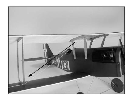
5. The rigging then will go from the front lower hole to the upper rear hole, crossing the outer strut.
