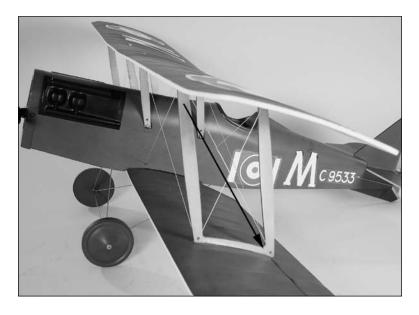
O 19. To complete the rigging of your model, go back and apply a drop of foam-safe CA to each position where the rigging passes through a strut and through the fuselage.
