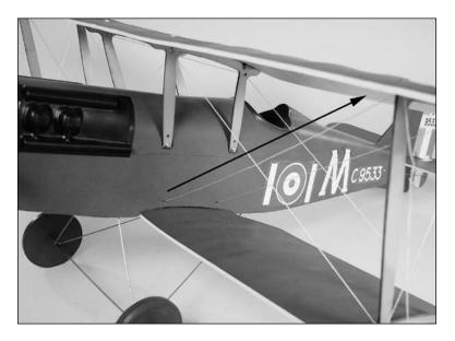
18. Apply light tension on all the rigging at this time. Use foam-safe CA to glue the end of the rigging in position once the rigging has been tensioned. Once again take a look and ensure there are no warps in the two wings. Using a hobby knife, trim off the remaining thread once the CA has cured.
