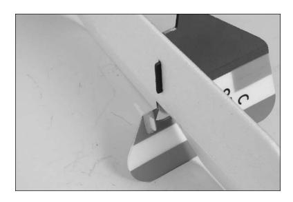
○ 4. Repeat Steps 2 and 3 to install the elevator control horn. The control horn faces down toward the bottom of the stabilizer/elevator.
