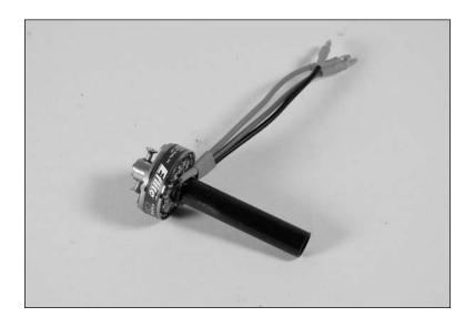
4. Lightly sand the motor tube once the adhesive used to glue the motor to the motor tube has fully cured.
