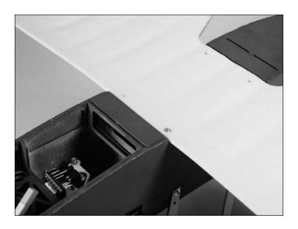
5. Using a ruler, check the alignment of the bottom wing to the fuselage. The distance from each wing tip to the end of the fuselage will be equal when the wing is in alignment. Move the wing as necessary to adjust the alignment until both measurements are equal.
