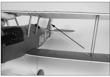
3. The rigging will then go between the two cabane struts.
