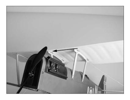
4. Route the rigging to the front lower hole in the outer strut as shown...
