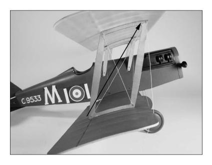
O 16. Run the rigging from the upper outer strut through the front tube in the fuselage.
