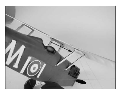
O 14. The rigging is then routed to the lower rear of the outer strut as shown.
