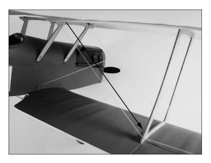
15. Next, route the rigging from the lower rear hole to the upper front hole in the outer strut.
