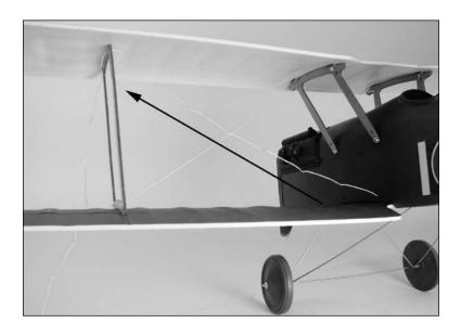
O 8. Cross the rigging from the rear upper hole back down the front lower hole where this section of rigging was started.
