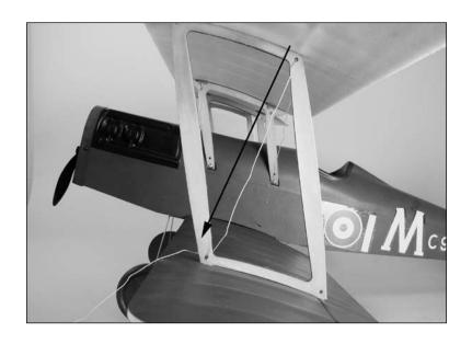
9. Apply light tension on all the rigging at this time. Use foam-safe CA to glue the end of the rigging in position once the rigging has been tensioned. Ensure you have not built a warp into the wings during this process. A quick sight from the front will verify there are not warps.
