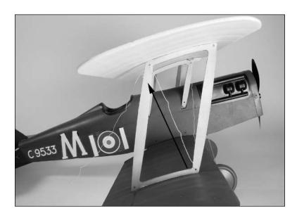
O 6. Route the rigging from the outer strut to the rear hole in the fuselage. This is where having a needle or hardening the rigging will come in quite handy.
