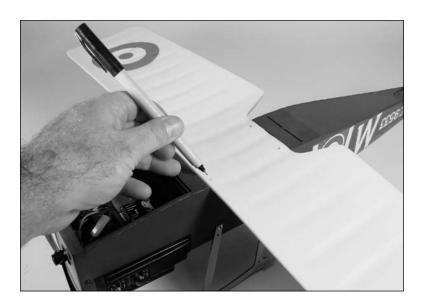
OOO 3. Use a pin drill and 1/16-inch (1.5mm) drill bit to drill a hole for the wing mounting screw marked in the previous step.
