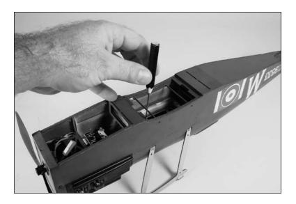
Phillips screwdriver to temporarily attach the wing to the fuselage. Using one screw will allow you to align the bottom wing as described in the following steps.
