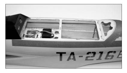
**Note**: You may want to tape off the fuselage around the cockpit opening for the next few steps to help protect the fuselage during the floor installation.
