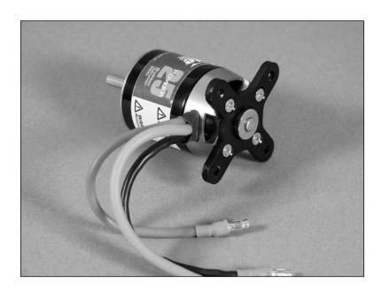
2. Attach the motor to the firewall using four 4-40 x 1/2-inch socket head screws, four #4 washers and a 3/32-inch ball driver. Make sure to use threadlock on the four screws to prevent them from vibrating loose.
