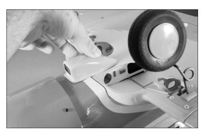
4. Attach the landing gear fairings to the wheel struts using two tie wraps per fairing. Use side cutters to remove the excess material from the tie wraps. Once the fairings have been attached with the tie straps, you can add a small drop of Medium CA to the inside to help secure it so it will not move in flight.
