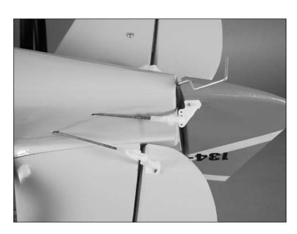
10. Slide the tail wheel onto the tail gear wire. Use a 1/16-inch wheel collar., setscrew and the included hex wrench to secure the wheel. Remember to use threadlock on the setscrew to prevent it from vibrating loose.
