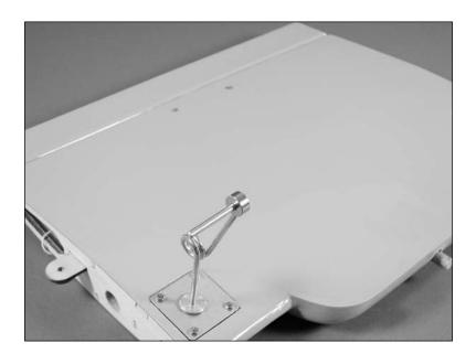
7. Slide the wheel onto the landing gear wire, then a final wheel collar. Use a 3mm x 4mm machine screw and #1 Phillips screwdriver to secure the wheel collar. Use threadlock on the screw to prevent it from vibrating loose.
