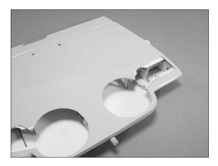
**Hint**: Trim the covering about 1/16-inch (1.5mm) from the inside edge of the opening and use a covering iron to seal the covering into the opening for a super clean retract installation.
