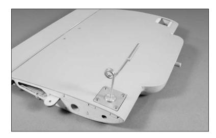
5. Use a file to create a flat on the bottom of the landing gear wire. This provides a place to tighten the screws for the wheel collars, making them more secure on the wire.
