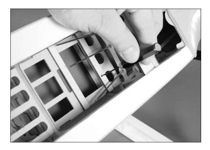
OOO5. Apply a few drops of thin CA to each of the holes drilled in the previous step to harden the surrounding wood.
