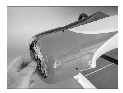
12. Use medium CA to glue the radiator scoop to the side of the fuselage behind the cowling. A felt-tipped pen can be used to color in the scoop to give that open look.
