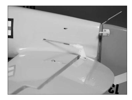
9. Slide a clevis retainer onto a nylon clevis. Thread the clevis onto the 21 <sup>3</sup>/<sub>4</sub>-inch (553mm) pushrod wire. Slide the pushrod wire into the opening in the fuselage that aligns with the stabilizer control horn. Snap the clevis onto the elevator control horn.
