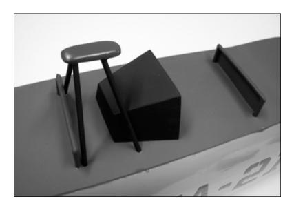
5. Glue the aft instrument hood in place using Medium CA. You will want to place the aft instrument decal from your kit on the panel at this time. Place the front instrument panel decal in place at this time.
