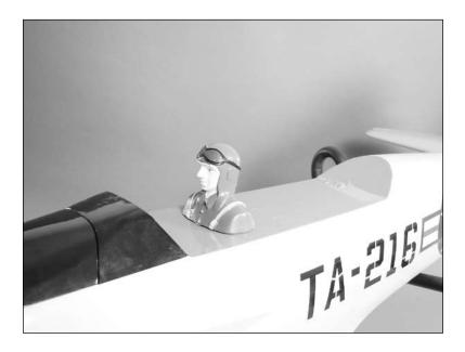
2. Use RC-56 canopy glue to attach the canopy to the fuselage. Use low-tack tape to hold the canopy in position until the glue fully cures. Note that the front of the canopy has a black strip that aligns with the antiglare panel on the front of the fuselage.
