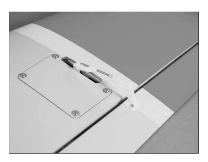
13. Secure a 6-inch (152mm) servo extension to the aileron servo lead and route it out the end of the wing panel.
