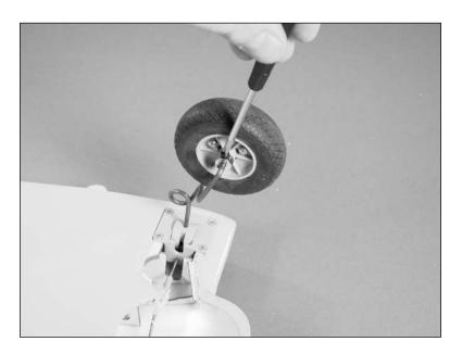
20. Check that the wheel is centered in the wheel well. Either bend the strut or change the position of the strut in the retract mechanism until the wheel is centered in the wheel well.
