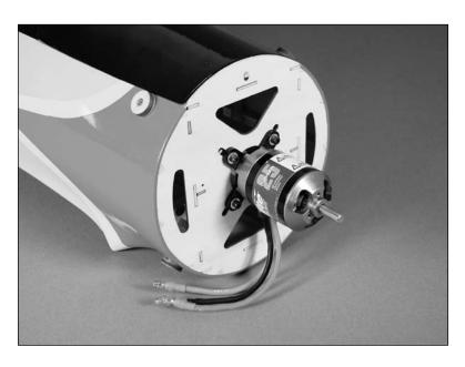
**Note**: The blind nuts in the fuselage for mounting the motor can be positioned for a variety of motors. Position them so they are aligned with your particular motor before mounting it to the firewall.
