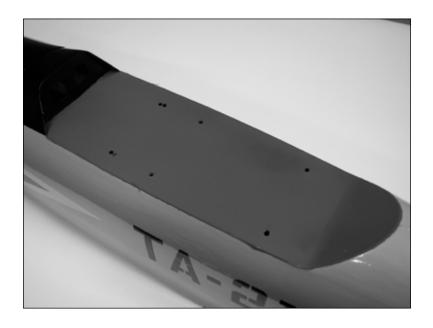
O 3. Glue the aft structure in place using Medium CA. You will want to make sure the canopy will fit on over the aft structure once in place and not cause any height issues.
