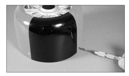
O 11 Slide the cowling back onto the fuselage and secure it using four 4-40 x 1/4-inch socket head screws and a 3/32-inch ball driver. Make sure to use threadlock on the screws to prevent them from vibrating loose.
