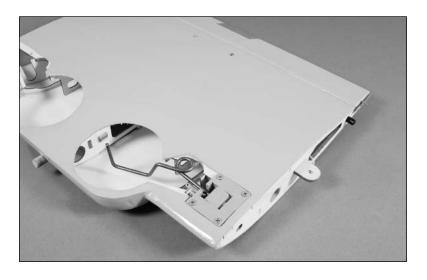
11. Slide a clevis retainer onto a nylon clevis. Thread the clevis onto one of the retract pushrod wires.
