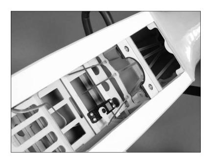
7. Repeat Steps 3 through 6 to install the remaining elevator servo and rudder servo.
