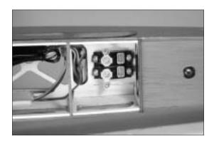
O 6. Insert the L-bend in the pushrod through the middle hole in the control horn.
