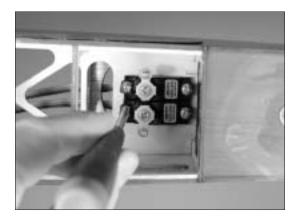
O 8. Pass the servo leads through the opening in front of the servos. Plug the servos into the receiver, making sure the rudder and elevator servos are in the correct channels. Plug the speed control into the receiver at this time too.
