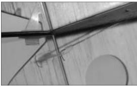
O 8. Use a ruler to center the elevator in the neutral position. With the radio system on, tighten the screw in the micro control connector to secure the pushrod wire at the servo.
