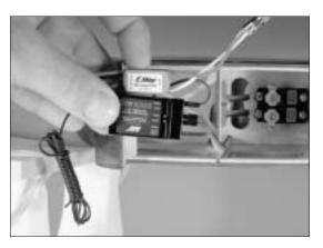
O 9. Use two-sided tape to mount the receiver and speed control to the sides of the fuselage.
