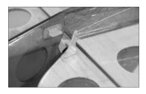
O 7. Slide the micro pushrod keeper onto the L-bend of the pushrod wire. The keeper then snaps onto the pushrod wire, securing the wire to the control horn.
