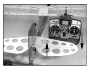
3. Use a ruler to adjust the throw of the elevator and rudder. Adjust the position of the pushrod at the control horn to achieve the flowing measurements when moving the sticks to their endpoints. Moving the linkage at the control horn can increase or decrease the throw. Moving the linkage to the top of the horn will decrease the throw, while moving toward the bottom of the horn will increase the throw.
