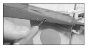
O 6. Use medium CA to glue the tailskid to the fuselage.
