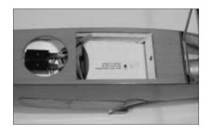
O 2. Place the battery hatch onto the fuselage. Use a 3/32" hex wrench to install the 4-40 x 1/2" screw and #4 washer.
