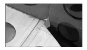
3. Repeat Step 2 for the rudder control horn. Note that the rudder control horn will be on the opposite side of the fuselage from the elevator control horn.
