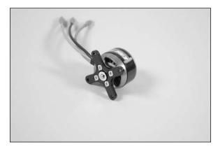
2. Attach the Outrunner motor to the front of the firewall using two plywood X-mount spacers, four #4 washers and four 4-40 x 5/8-inch socket head screws. Tighten the screws using a 3/32-inch ball driver or hex wrench.
