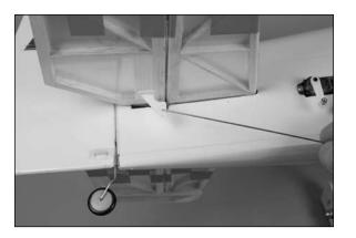
OO 13. With the radio system on, make sure to center the elevator trim and stick. Make sure the elevator servo is operating properly using the transmitter. Slide the pushrod wire through the micro connector on the servo horn. Center the elevator, and secure the position of the wire using the 2mm x 4mm screw and a #0 Phillips screwdriver.
