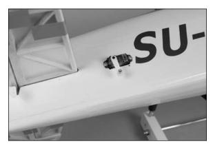
○○ 8. Insert the bend in the 4<sup>1</sup>/<sub>2</sub>-inch (115mm) pushrod wire into the middle hole of the elevator control horn.
