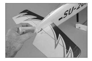
• 12. Firmly grasp the stabilizer and gently pull on the elevator to ensure the hinges are secure and cannot be pulled apart. Use caution when gripping the elevator and stabilizer to avoid crushing the structure.
