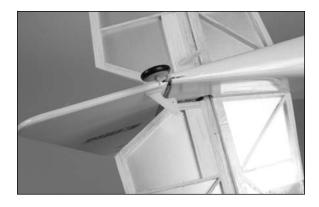
14. Slide the micro control horn backplate on the control horn from the opposide side of the rudder as the control horn. Apply 2–3 drops of thin CA at the joint between the horn and backplate to keep it secure.
