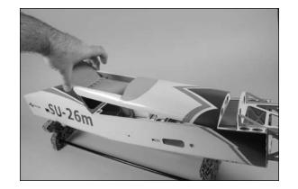
OO 2. Slide the landing gear in the slot in the side of the fuselage. Secure the landing gear using two 4-40 x 1/2-inch socket head screws and two #4 washers. Use threadlock on the screws before tightening them with a 3/32-inch hex wrench or ball driver.
