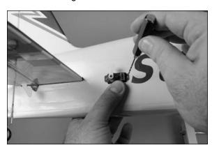
OO 3. Apply 2-3 drops of thin CA into each of the two holes to harden the surrounding wood.
