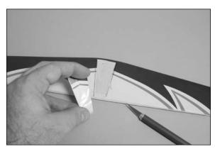
• 6. Insert the micro control horn into the slot in the elevator. Make sure the holes in the control horn face forward and that the horn is on the side with the clear covering (bottom).
