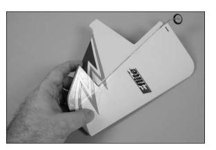
• 10. Place the fin in position on the fuselage. Trace the outline of the fuselage onto both sides of the fin using a felt-tipped pen.
