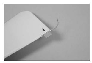
• 4. Slide the tail wheel onto the wire. The wheel is then secured using the tail wheel keeper and a drop of thin CA.
