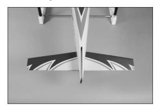
• 2. View the airframe from the rear and make sure the wing and stab are parallel. If not, lightly sand the stab saddle until they are.
