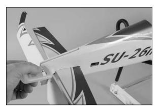
• 10. Slide six hinges into the slits in the elevator. Place a T-pin in each hinge to prevent it from being pushed into the elevator when attaching it to the stabilizer. Slide the elevator tight against the stabilizer.
