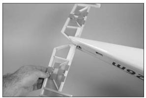
9. Check the alignment and make sure everything lines up. Wick thin CA into the joint between the fuselage and stabilizer. Make sure to glue both top and bottom. Do not use accelerator—to allow the CA to wick in the joint, providing the best bond possible.
