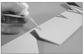
$\mathbf{O}$  ~ 8. Slide the elevator into position, then the stabilizer.  $\mid \mathbf{O}$
