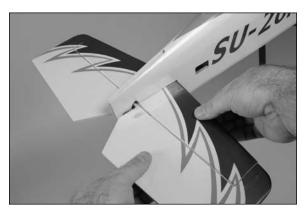
13. Work the elevator up and down several times to work in the hinges and check for proper movement.
