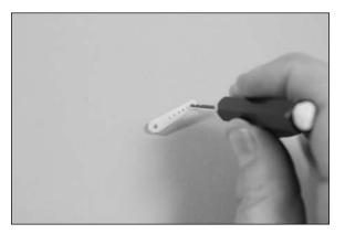
**OO** 6. Attach the micro control connector to the servo horn. Be sure to use the included retainer to secure the micro control connector.
