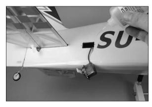
••• 4. Use a #0 Phillips screwdriver and the screws provided with the servo to secure the elevator servo in the fuselage.
