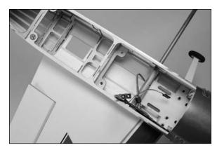
• 4. Repeat Steps 2 and 3 to attach the remaining wing panel to the fuselage.
