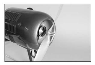
• 6. An optional  $1^{3}/_{4}$ -inch spinner is also available for your model. It can be installed at this time.
