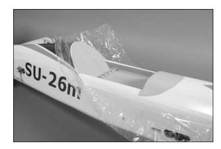
• 4. Use canopy glue to secure the canopy to the hatch. Use low-tack tape to keep the canopy in opposition on the fuselage until the glue fully cures.
