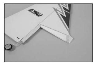
• 12. Position the fin back onto the fuselage. Use a square to check the alignment between the fin and stabilizer. Lightly sand the bottom of the fin until the alignment is correct. Use thin CA to glue the fin to the fuselage. Also apply CA to the rudder post at the back edge of the fuselage.
