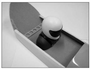
• 3. Place the canopy hatch on the fuselage. Make sure to place a piece of waxed paper or part of a bag from the packaging of your model between the hatch and fuselage so when the canopy is glued to the hatch it won't accidentally be glued to the fuselage. Make sure that the hatch is fully seated on the fuselage, and the magnet in engaged during this step. If it is not seated and engaged, it could cause your hatch to fit improperly or not engage once the canopy is glued on.
