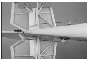
• 15. Use hook and loop tape to mount the receiver and remote receiver in the fuselage. Plug the elevator, rudder and speed control leads into the appropriate ports of the receiver.
