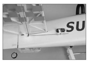
• 14. Repeat Steps 1 though 13 to install the rudder servo and linkage. The linkage will also connect to the center hole of the rudder control horn and to the outside hole of the 3D servo horn.
