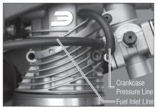
1. Connect medium diameter tubing to the carburetor and the fuel tank supply line.
