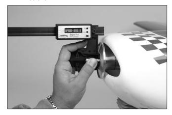
Attach the thrust attachment to the prop hub carefully without upsetting the position of the airplane and record the relative thrust angle
