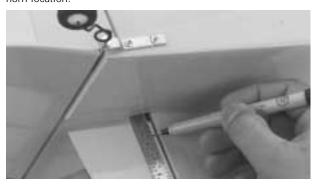
**Step 2.** Place the center of the control horn on the elevator at the mark made in the previous step. Mark the hole positions of the control horn with a felt-tipped pen or pencil.
