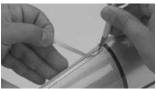
**Step 11.** Re-install the fin into the fuselage to check the fit.
