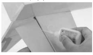
**Step 9.** Once the CA has dried, check the hinges for security by trying to pull the elevators from the stabilizer. Use only slight pressure and be sure not to crush the wood structure of the stabilizer or elevator.
