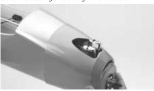
**Step 2.** Looking at the firewall, notice the plywood doubler on both sides of the fuselage. Measure 1/2" from the top and bottom of the doubler and mark with a felt-tipped pen, marking both sides of the fuselage. Measure 3/8" back from the firewall at the four marks you just made and make a mark. These are the cowl mounting screw locations.
