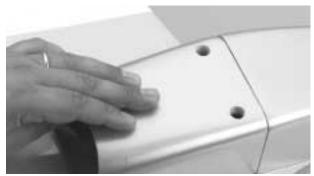
**Step 8.** With the radiator scoop properly positioned, use a pencil to trace the outline onto the wing. Use only enough pressure to make a slight indentation in the covering. Use a sharp hobby knife to cut away the covering 1/16" inside the line you just made.
