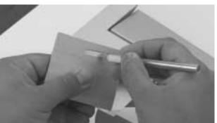
**Step 2.** Install the recommended servo hardware (grommets and eyelets) supplied with your radio system onto the aileron servo. Temporarily install a long half servo arm (JRPA212) onto the servo and test fit the servo to the hatch. The servo output shaft and control arm should be centered in the slot of the hatch. Once satisfied, mark the location for the servo mounting blocks.
