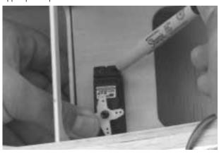
**Step 7.** Remove the throttle servo and drill the screw holes you just marked with a 1/16" drill bit.
