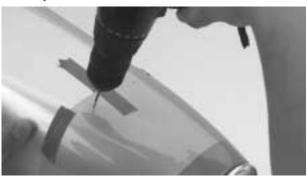
**Step 7.** Mount the cowl using the #2 wood screws provided.
