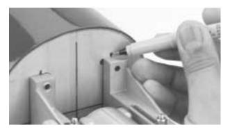
**Step 3.** Install the 8-32 blind nuts from inside the fuselage and mount the rails to firewall. Seat the blind nuts by tightening the bolts. Remove the bolts and carefully glue the blind nuts in place with Thin CA, be sure not to get any CA on the threads of the blind nuts.
