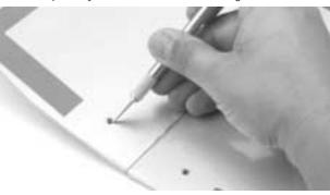
**Step 3.** Locate the plywood wing mounting plate. Align the plate with the trailing edge of the wing and the center joint as shown and mark the outline of the plate with a felt-tipped pen/pencil. Use a sharp hobby knife to trim away the covering 1/16" inside the lines you just drew.
