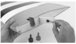
**Step 8**. Carefully slide both wing panels together. Firmly press both halves together, allowing the epoxy to run out. Use alcohol and paper towels wipe off the excess epoxy. Check to make sure there are no visible gaps between the two wing panels.
