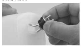
**Step 8.** Tighten the 3mm screw carefully—do not over tighten. This allows the rubber stopper to form a seal by being slightly compressed, thus sealing the fuel tank opening.
