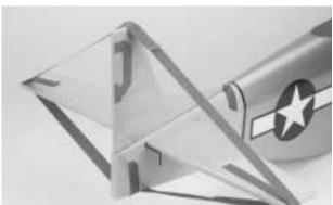
**Step 15.** Double-check the alignment of the horizontal stabilizer and vertical fin and use masking tape to secure it in place. Use rubbing alcohol and paper towels to clean the epoxy off of the elevator joiner wire. Allow the epoxy to fully cure.
