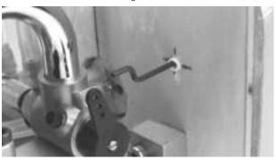
**Step 9.** With the throttle stick centered move the throttle arm on your engine to the center of its throw (1/2 throttle) and tighten the setscrew on the EZ connector. Trim off the excess wire.
