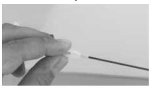
**Step 2.** Attach one clevis to the rudder control horn and, with the rudder centered and the servo electrically centered, mark the wire where it passes over the outermost hole on the servo arm.
