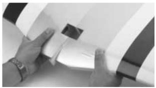
**Step 3.** Check for correct dihedral angle. Place the wing on a large flat surface with one wing panel resting flat on the surface the opposite wing panel should be  $5^{1}/4^{\circ}$  from the flat surface (see illustration below). If necessary, sand the wing joiner until the proper dihedral is achieved. There should be no gap at the wing center joint. Once you are satisfied with the fit, separate the wing panels and remove the wing joiner.
