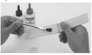
**Step 6.** Apply a generous amount of epoxy to the other wing panel joiner cavity.
