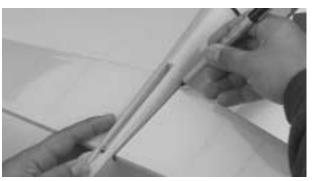
**Step 7.** Remove the stabilizer and use a sharp hobby knife to carefully remove the covering from the center of the stabilizer, cutting 1/16" inside the lines you marked in the previous step. Use only enough pressure to cut the covering and not the wood underneath, as doing so will severely weaken the structure of the horizontal stabilizer.
