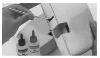
**Step 7.** Apply epoxy to the exposed portion of the wing joiner and to both wing roots.
