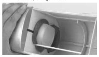
**Step 6.** Test fit the throttle pushrod tube through the firewall and into the fuselage. Once satisfied with the fit, mix 1/4 ounce of 6-minute epoxy and glue the pushrod into the firewall. Allow the epoxy to cure.
