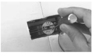
**Step 11.** Cycle the retract system several times and check to make sure there is no binding, also check that the landing gear locks in both the retracted and extended position.
