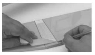
**Step 8.** Re-install the stabilizer into the fuselage. Use the lines drawn in Step 6 to reposition the stab correctly. Looking from behind the plane, check to make sure the horizontal stabilizer is parallel to the wing as shown in the illustration below. If any adjustments are require lightly sand the stabilizer saddle to bring the horizontal stabilizer into alignment with the wing.
