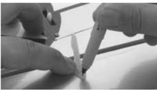
**Step 4.** With the mounting hole locations marked, drill the holes for the mounting screws using a 1/16" drill bit. Be sure to drill straight through the aileron at a 90-degree angle to the flat work surface not to the surface of the aileron.
