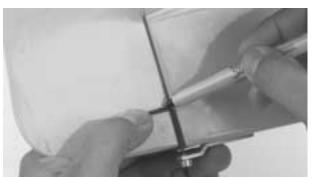
**Step 3.** Using a 3/32" drill bit, drill the rudder following the marks you made in the previous step. Make sure to drill straight into the rudder.
