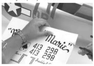
**Step 5.** Use the drawings to locate the position of the decals on the P-51. Use a water spray bottle with 2-3 drops of dish soap added to the water and spray both the fuselage and sticky side of the decal. This will allow you to reposition the decal if necessary. Once satisfied with the position use a paper towel to squeegee out the water. Allow the decal to dry over night.
