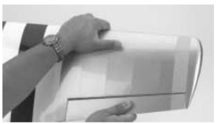
**Step 9.** Work the aileron up and down several times to "work in" the hinges and check for proper movement.
