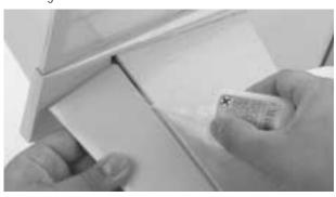
**Step 8.** Turn the fuselage over and repeat the hinge gluing process by deflecting the elevators in the opposite direction and again completely saturating each hinge with thin CA. Wipe away any excess CA using CA Remover/Debonder and a paper towel. Allow the CA to completely dry.
