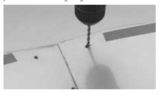
**Step 6.** Mount the wing to the fuselage using the two provided mounting bolts and washers. Tighten the bolts finger tight and align the wing to the fuselage by measuring from the wing tips to the center rear of the fuselage as shown. The measurements should be equal on both sides. It may be necessary to enlarge the holes in the mounting plate to get the proper alignment.
