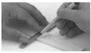
**Step 2**. Trial fit the wing joiner into one of the wing panels. It should insert smoothly up to the line marked in Step 1. Now slide the other wing panel onto the joiner until the two panels meet. If the fit is too tight, it may be necessary to lightly sand the wing joiner.
