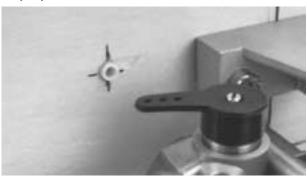
**Step 5.** Determine the proper location for the throttle pushrod. Mark the location with a felt-tipped pen or pencil and drill the firewall for the pushrod tube using a drill and 1/8" drill bit. Remove the engine if necessary.
