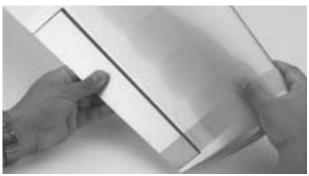
**Step 4.** Deflect the aileron and completely saturate the hinge with thin CA glue. Be sure not to deflect the aileron too far; the top of the aileron should just touch the top of the wing trailing edge. When the hinge is glued in place, there should be no more than a 1/32" gap maintained throughout the length of the aileron.
