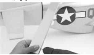
**Step 3.** Temporarily install the elevators back onto the horizontal stabilizer and check for fit. The elevator halves should be equal to each other and move freely up and down. If the elevators are not equal, you can remove them and carefully bend the joiner wire until they come into alignment. Once satisfied with the fit, remove the elevator halves.
