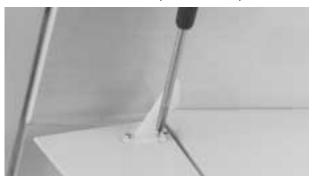
**Step 5.** Measure  $1^{1}/_{2}$ " up from the bottom of the rudder on the left side of the rudder. Mark the location with a felt-tipped pen or pencil. This mark will serve as the center for the rudder control horn.
