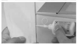
**Step 10.** Once the CA has completely dried, check the rudder for security by trying to pull the rudder from the fuselage. Use only enough pressure to test for security and be careful not to damage the wood structure of the rudder or fin.
