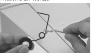
**Step 2.** Temporarily install the rudder using the hinges provided; do not glue the hinges at this time. Hold the tail wheel assembly up to the fuselage as shown and mark the location where the wire will insert into the rudder. Remove the rudder.
