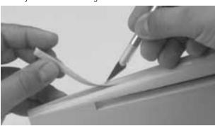
**Step 2.** Locate the horizontal stabilizer and elevator assembly and remove the elevators and hinges. Use a felt-tipped pen or pencil and ruler to mark the center of the stabilizer at the trailing edge as shown.
