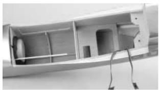
**Step 6.** Temporarily install the throttle servo as shown with the output shaft to the side of the fuselage where the pushrod is located. Mark the mounting screw hole locations with a felt-tipped pen or pencil.
