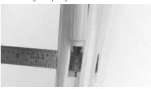
**Note:** The horizontal stabilizer is positioned all the way forward in the saddle area to allow room for the elevator joiner wire. The wire will be inserted through the saddle area before the horizontal stabilizer is glued in place.
