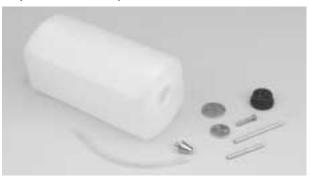
**Note:** The stopper provided with the P-51 has three holes hat are not bored completely through the stopper. You will only be using two holes: one for the fuel pickup and one for the fuel vent. Make sure not to open the third hole, as this will cause a fuel leak.
