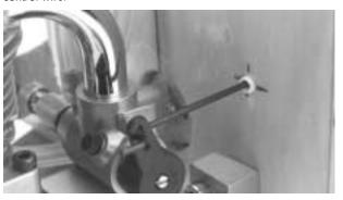
Check the throttle movement and adjust the end points if using a computer radio. If using a non-computer radio, adjust the end points by moving the connection of the wire either closer or further away from the center of the servo or throttle arm.
