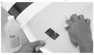
**Step 9.** Use masking tape to securely hold both wing halves together. Place the wing assembly back onto the flat work surface (covered with wax paper), and check the dihedral again as in Step 3.
