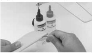
**Step 8.** Install the rudder and wipe away excess epoxy using rubbing alcohol and paper towels. Remove the T-pins and move the rudder against fin until there is only a slight gap (1/32" or less). Use masking tape to secure the rudder to the fin and allow the epoxy to cure.
