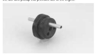
**Step 3.** Slide the smaller of the two caps over the tube on the smaller end of the rubber stopper. The small end will be inserted into the fuel tank. The larger cap is placed on the other side of the rubber stopper that makes the cap. Loosely install the 3mm screw through the stopper.
