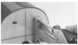
**Step 4.** Install the engine mount rails using threadlock and the 9/64" hex wrench. Loosely mount the engine to the rails and measure 5<sup>1</sup>/<sub>4</sub>" from the firewall to the prop drive washer of the engine. Tighten the mounting hardware and mark the location of the engine on to the mount. Use these marks to properly position the engine if it needs to be removed in the future.
