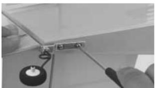
**Step 6.** Install the rudder hinges placing a T-pin through the center of each hinge to keep it centered while installing the rudder.
