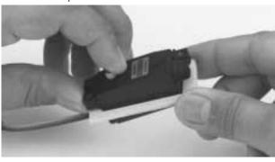
**Step 3.** Mark the location for the servo mounting screws using a felt-tipped pen or pencil. Remove the retract servo from the mounting plate and using a 1/16" drill bit, drill the holes for the servo mounting screws. Temporarily mount the retract servo to the mounting plate using the screws supplied with the servo.
