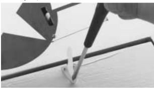
**Step 7.** Remove the clevis and wire from the control horn and make a 90-degree bend at the mark made in the previous step. Cut off the excess wire leaving 5/16" remaining after the 90-degree bend.
