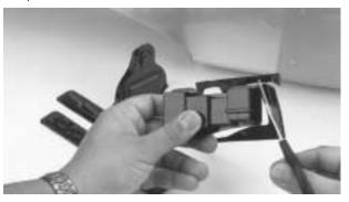
**Step 2.** Using the detail drawings, glue the cockpit detail to the fuselage using Shoe Goo or similar type adhesive. Secure the parts with tape until the glue has dried.
