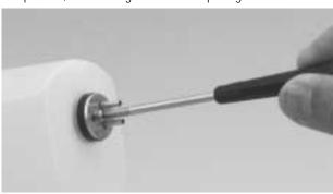
**Important:** Be sure to differentiate between the vent and the fuel pick-up tube. Once the tank is mounted inside the fuselage, it will be difficult to tell the tubes apart.
