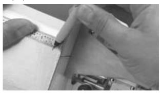
**Step 3.** To transfer these locations to the cowl, tape a piece of paper to the side of the fuselage as shown. Transfer the screw locations to the paper and fold back along the tape line.
