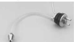
**Step 7.** Carefully insert the assembly into the fuel tank. Note the position of the vent tube; it must be at the top portion of the fuel tank to function properly. Also, it may be necessary to shorten the length of the fuel pickup tubing to make sure the clunk does not rub against the back of the fuel tank. You should be able to turn the tank upside down, which allows the clunk to freely drop to the top of the tank.
