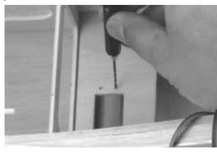
**Step 8.** Mount the throttle servo using the screws provided with your radio system. The throttle linkage will be installed later in this manual.
