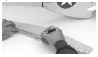
**Step 3.** Mark the center of the stabilizer saddle at the trailing edge of the saddle. You can hold the ruler at the back portion of the stab opening and use a pen or pencil to mark the center location through the opening of the vertical fin as shown.
