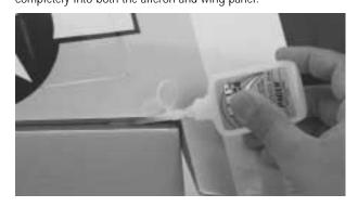
**Step 6.** Using CA remover/debonder and a paper towel, remove any excess CA glue that has accumulated on the wing or aileron surface.
