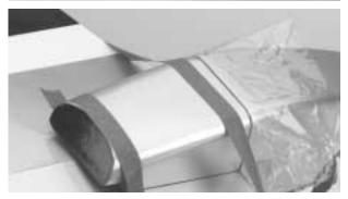
**Step 10.** Once the epoxy has cured remove the wing and use a 1/4" piece of fuel tubing over the mounting bolts to keep them from falling out.
