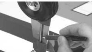
**Step 7.** Turn the fairing over and draw a line from the top to the bottom. Measure in 2" from both the top and the bottom and mark the location for the mounting straps.
