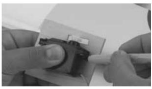
**Step 3.** Locate the servo mounting blocks. Using a few drops of thin CA, tack glue them in place on the marks made in the previous step. Check the fit of the servo between the mounting blocks. When satisfied with the fit, permanently glue the mounting blocks in place by first wicking thin CA between the mounting blocks and the hatch, and then using thick CA create a fillet around the base. Let the CA completely dry before proceeding to the next step.
