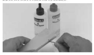
**Step 6.** Install each elevator onto the hinges and the joiner wire. Remove the T-pins and push the elevators close to the stabilizer until there is only a slight gap (1/32" or less) at the hinge line. Wipe away any excess epoxy with rubbing alcohol and paper towels. Use masking tape to hold the elevators in place and allow the epoxy to cure completely before moving to the next step.
