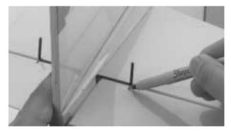
**Step 2.** Remove the elevators. Using a 3/32" drill bit, carefully drill the holes into the elevators using the marks you made in the previous step as a guide. Drill directly down the center of the elevator and only as far as needed.
