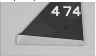
**Note**: Use care not to cut into the underlying wood and weaken the structure. Doing so could cause the fin to fail in flight, resulting in the loss of your airplane.
