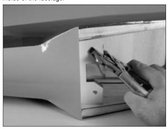
**Note**: Make sure no epoxy gets into the threads of the blind nut.
