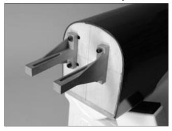
**Hint**: You can also install the blind nuts backwards to prevent them from pulling into the wood on the backside of the firewall. Just remember to move them to their correct positioning before moving to the next section.
