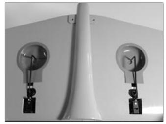
**Hint**: Use clear tape and tape the wells into position when flying from rough surfaces. This will allow easy access to the linkages in case they might need future adjustments.
