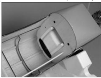
**Note**: Make sure that any support braces installed will not interfere with the installation of the wing or linkages.
