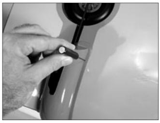
☐ ☐ **Step 13**Secure the gear fairing to the wing using eight 2mm screws.
