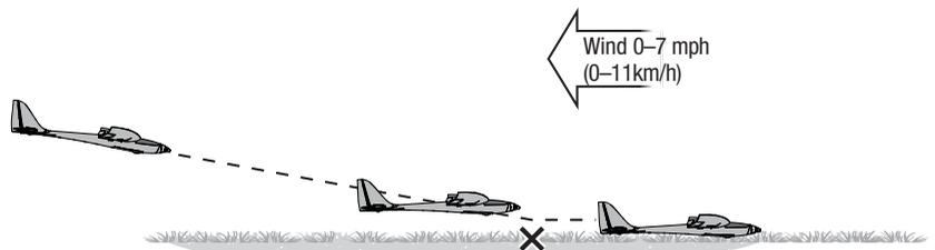
**NOTICE:** If a crash is imminent, reduce the throttle. Failure to do so could result in extra damage to the airframe, as well as damage to the receiver and motor.
