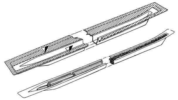
Re-fasten the central part to the hull and place it upside down. Draw the dimensions shown on the hull and glue the keel along the centre line to the hull. Let everything dry well. The edge of the facing area
