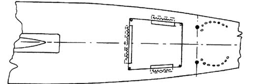
Then you apply scrap pieces to the lid, as per the drawings below, so that it can be hooked up and clamped in like the stern hatch.
