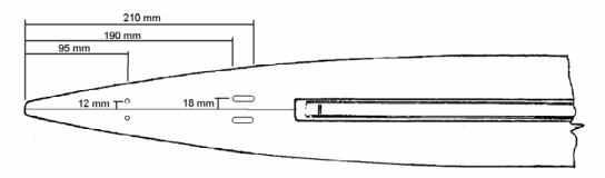
Use a straight edge for attachment and place it vertically at the stern. For drilling the two holes for the rudder tubes first use a 2mm drill bit, then open it up to 4mm. For the space for the stern tubes, we also recommend starting off drilling the end point with a small drill bit and gradually opening it up to 7mm and filing it.
