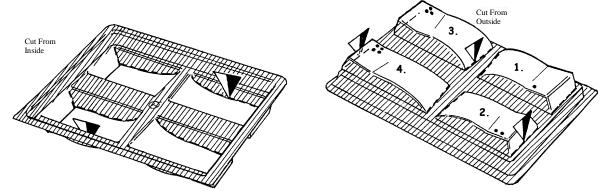
Now cut out the 4 cover fastening braces. For this, first cut along the wavy lines from the inside and then the cross lines from the outside. The parts are marked with dots from 1 to 4.
