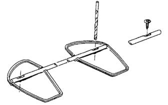
Glue the half rudders together and let them dry. Check the alignment of the fins by placing them on a level surface. Carefully sand the glued edges.
