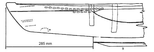
Now measure and mark all other parts cut out from the build plan and the following drawings and mark these dimensions on the hull.
