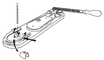
Then turn the form part around and cut out the tower deck from the inside. Repeat this with the inner frame (69) and use a small round file to work out the semi circular apertures. Drill 4 x 3mm holes in the raise for the periscope in the middle of the deck.
