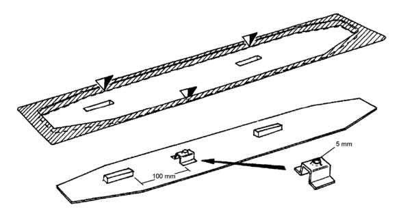
At the same place in the upper part, drill a 5mm hole for the ventilation pipe. Glue the pipe into the upper shell and holder using epoxy adhesive and simultaneously glue the floor with ABS adhesive into the upper part. Cut off the edge of the upper part and sand it level with the floor. Drill a 5mm hole each fore and aft into the front very close to the floor for the connection pipes (56) and glue these into place.
