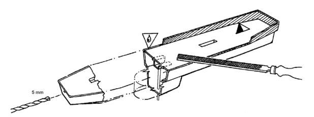
Now drill 8 small holes of 2mm diameter around the ventilation pipe and one each fore and aft into the tower roof of the flood tank.
