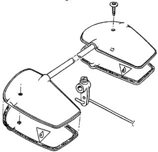
After a piece of tubing (39) and a set collar (38) have been pushed on, the wire (37) can be pushed into the inner tube of the Bowden cable. Please consult the build plan for this step. The adjustment is carried out later.
