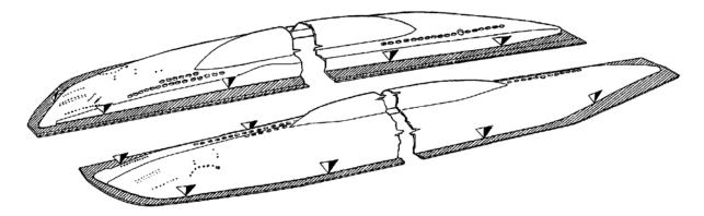
Using first fine and then coarse sanding paper, sand the flood apertures that are raised from the inside and the details. Sand down to the wall. When building the display models, we also recommend sanding the apertures, but unlike in the powered model where they are to remain open, they are then closed again from the rear using a black lacquered component. This, in our view, makes the apertures look tidier rather than just leaving them closed and only painting them over.
