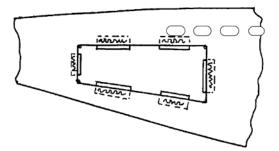
Cut out 3 strips for the cover which you then glue vertically to the inside of the cover. The cover should then be hooked in with its upper edge into the hull and slot into the lower edge by lifting it up and over.
