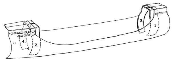
Fixing with nuts and bolts: Set the central part back on the hull and hold it with adhesive tape. Drill 4 holes of 3 mm diameter through the central part into the braces. Remove the central part again.
