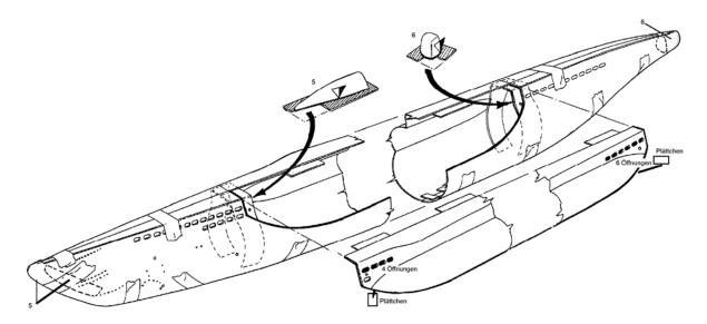
Now put some ABS glue on the 5 linking pieces of the central part and re-insert the backboard central part. Let the adhesive dry.
