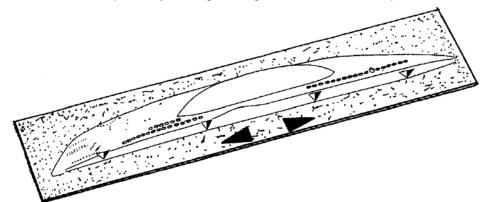
Bend some strips of  $12 \times 1.5$  mm ABS so as to follow the contours of the hull radius. Cut these into 40 pieces of 25 mm length each (3). They will be glued to the interior of the lower hull half.
