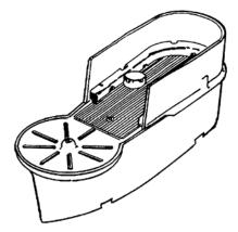
Drill 6 x 3mm holes from below into the deck (but not into the inner step) so that they are not visible from the outside. Glue the compass part (68) into place.
