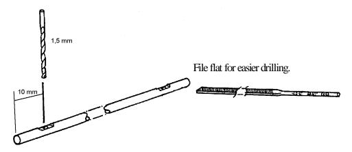
Drill through the half fins with the ends of the shaft positioned right on the outside.
