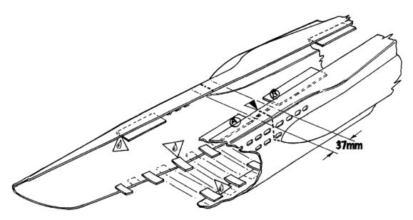
Start by gluing 20 bent strips (3) in the area of the floor onto each hull half at a distance of ca. 35 mm between each component, so that they interlock with each other.
