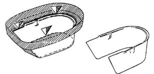
Cut out the lower tower part - below from the inside and above from the outside. The illustration shows it upside down.
