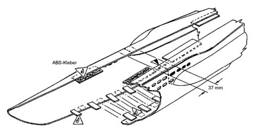
Once dry, sand down the overlapping glue with wet sanding paper until the connecting edge is smooth. Any gaps can now be filled with plastic putty. You can also make your own putty in a small jam jar with ABS adhesive and ABS chippings. However, it will take some time until the plastic has dissolved in the glue enough so that it can be used.
