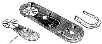
Sand the edges until the deck fits cleanly into the lower tower part. Now glue it into the tower and let it dry. File the edge down to deck level but be careful that you do not file any detail. Cut apertures into the floor of the lower tower part 4 as shown.
