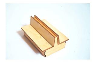
On the side of the flybridge wall sand the protruding parts of the bolsters flat.
