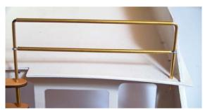
Make the end piece at the left ladder rod from a piece of brass tube 2 x 7 mm (104) and glue.
