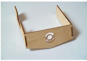
Now make the battery and receiver tray with parts 19, 20 and 21.
