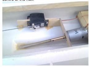
Now fix the tube and the motor mount with UHU Plus Acrylit inside the hull and fill the end of the hull around the shaft with glue that it is water tight.
