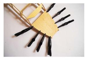
When the glue is dry, do the same on the other side. After that, glue from inside and fix with clamps.
