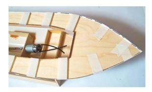
Fix the deck at several points with thin superglue. After that you can fix the deck complete with medium superglue. A good help is also Activator spray to shorten the drying process.
