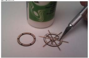
Apply some glue to the outer ring and into the center of the wheel and plase the spokes carefully that they are lying up to the center hole, but leave it free.
