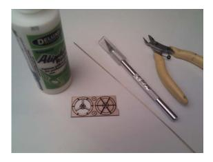
For this assembly fo the steering wheel you will need the small laser sheet, 12 cm of brass wire 1 mm, and white glue or Aliphatic glue, a modelling knife, a wire cutter and some sand paper.
