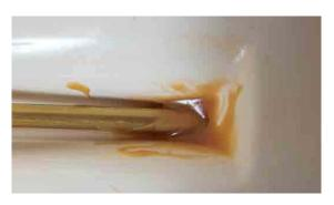
After the glue is set, you can also fix the rudder shaft in the same way.
