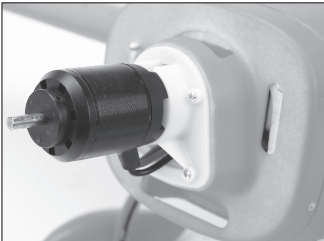
View of the motor on the motor mount
