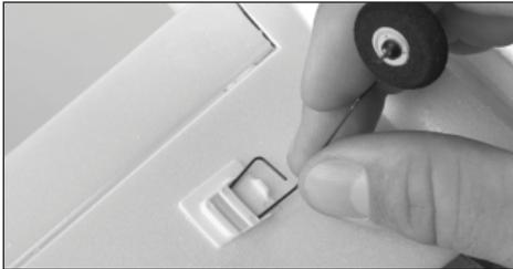
2. Gently slide left and right mainlanding gear into plastic mounting clips on the bottom of the wings, orienting the struts toward the front of the airplane as shown.
