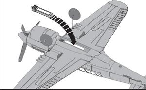
Connect the battery to the ESC, noting proper polarity.
