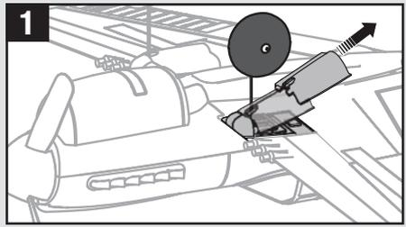
2. Lift the end of the landing gear wire above the stop.
