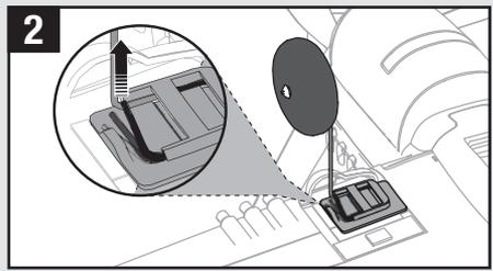
3. Gently pull the landing gear away from the fuselage and away from the clips.
