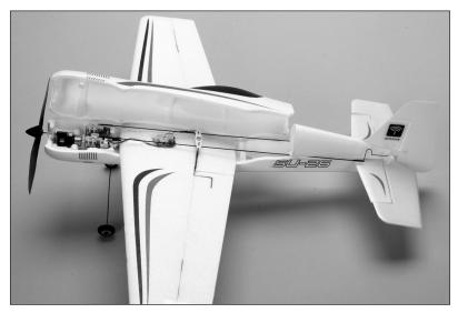
The servo pushrod is in the outer hole of the aileron bellcrank.
