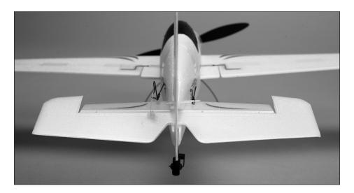
When the elevator stick is moved aft the elevator should move up.
