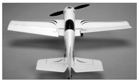
Move the rudder stick left and right to check yaw control. When the stick is pushed to the right the rudder should also move to the right (if viewed from behind the airplane).
