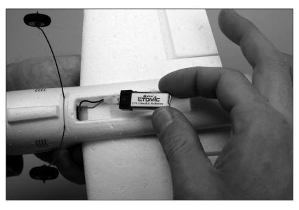
Note: The battery cavity is oversized to allow for the Center of Gravity adjustment. Start with the battery in the middle of the battery cavity. Adjust the battery forward or rearward to fine-tune the CG.
