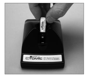
Gently press the battery and its connector into the charge jack/ connector located at the bottom of the slot in the charger. Again, be
