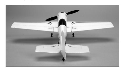
With the rudder stick pushed to the left, the rudder should move to the left (if viewed from behind the airplane).
