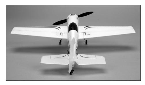
If at any time during the test the controls respond in the opposite direction, it may be necessary to reverse/change the direction of operation of the flight controls. Follow your transmitter instructions to change the direction of the various flight controls.
