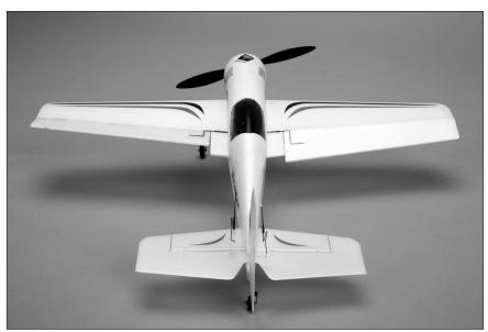
With the aileron stick pushed right, the right aileron should move up and the left aileron should move down.
