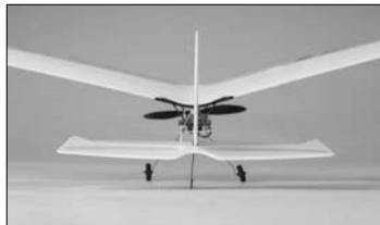
5. Pull the right stick back and the elevator control surface should move upward.
