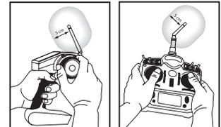
The following illustrations show the approximate 5 cm RF exposure area and typical hand placement when operating your Spektrum transmitter.
