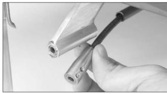
☐ 3. Remove the drive shaft flex cable. Replace the Teflon liner as needed.
