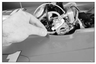
Close the choke by rotating the small yellow tubing extension. This is not necessary if the engine is warm.
