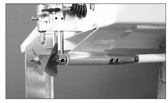
□ 5. Reassemble in reverse order. Make sure the setscrews are tightened down on the flat spots of the prop shaft. Also be certain to place a drop of threadlock on each setscrew before retightening them.
