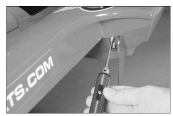
□ 5. Carefully attach the turn fin onto the right sponson as shown and tighten the hex screws with a 3mm hex driver.
