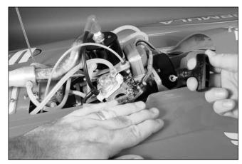
With an assistant holding the boat to the boat stand and bracing the engine with one hand, pull the starting cord briskly several times. Once the engine fires (begins to start), open the choke. Prolonged choking will flood the engine with fuel. See Section 15: Troubleshooting Guide to correct the flooding condition.
