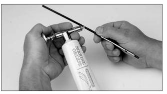
☐ 4. Lubricate the entire flex cable with waterproof grease (PRB0100) as shown and then reinstall the flex cable back through the liner and stuffing box and into the clutch.
