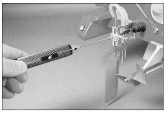
□ 3. Find the flat spot on the rudder. Put screw locking compound on the 2.5mm hex screw threads and tighten the screw on the flat spot as shown.
