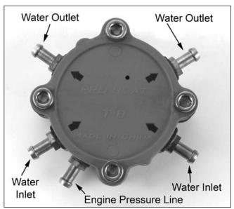
The water pump is operated from crankcase pressure. Be sure that water is exiting the 2 water jackets mounted on the left side of the boat when the engine is running and the boat is in the water. If water does not stream out of either the exhaust or cylinder head cooling ports, immediately stop engine operation and remove obstructions in the lines or replace broken cooling lines.
