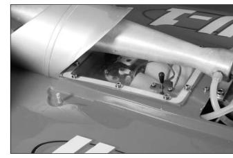
☐ 3. Plug the switch harness into both the receiver and the battery box following the instructions provided with the radio. Secure the radio box cover with the hex head screws.
