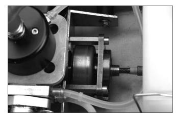
The centrifugal clutch automatically engages when the engine rpm is increased. Be sure the idle speed adjustment is set low enough so that the propeller does not rotate at idle.
