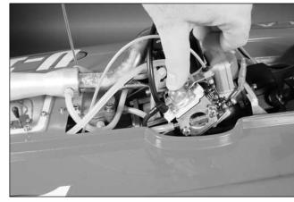
Press the priming bulb several times until it becomes filled with fuel. This is not necessary if the engine has recently been run.
