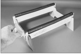
□ 2. Secure the interlocking boat stand with medium thick CA or epoxy. Make certain you allow the CA or epoxy to fully cure before placing the boat on the stand.
