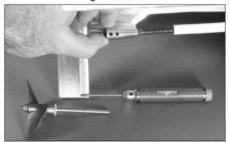
□ 2. Loosen and remove the two 2.0mm set screws that secure the propeller shaft to the brass ferrule. Remove the prop drive dog and nylon washer.
