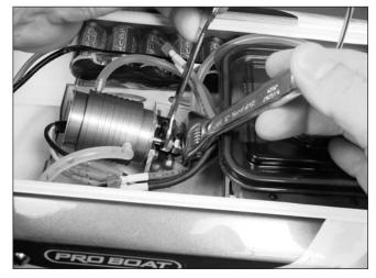
• 2. Remove the hex screws holding the prop strut in position. Remove the entire assembly with the flexshaft.
