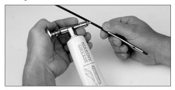
Carefully reinstall the drive shaft, making certain that there is a 1–2mm gap between the prop strut and the drive dog to allow for flexshaft shrinkage under load.
