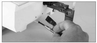
Wipe off all dirt or debris from the flexshaft and liberally lubricate the entire length of the drive shaft with silicone cable grease.
