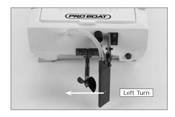
The ESC will beep until you give full throttle input. The auto sensing circuitry will select full throttle position when you hold full throttle during initial setup. Release the throttle trigger. With the propeller free from any objects, give some throttle input to ensure that the motor is working. If everything appears to be functioning correctly, you are ready to run your boat!
