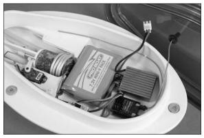
O 10. Confirm that the ESC on/off switch is in the "OFF" position and connect the battery to the battery plug from the speed control.
