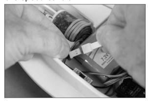
O 11. Turn on the transmitter, then the ESC on/off switch. The radio system is now searching for the receiver it is bound to. Once located, the LED on the receiver will illuminate and allow rudder operation.
