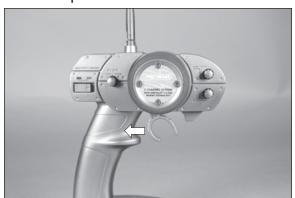
O 12. Check the operation of the steering in relationship to the steering wheel. When the wheel is rotated clockwise, the thruster must move right as shown. If not, follow the instructions from the radio to set the servo reversing for the steering. You may increase or decrease the amount of steering authority by adjusting the Steering Dual Rate (S.T. D/R) on the transmitter.
