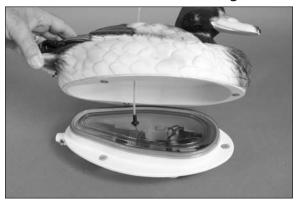
O 7. Remove the radio box cover from the hull by lifting it up and away from the hull.
