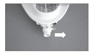
O 13. Place the clear battery cover back into position. Be sure the longer antenna wire is extended through the antenna tube and the short antenna wire is clear of any moving parts inside the hull.
